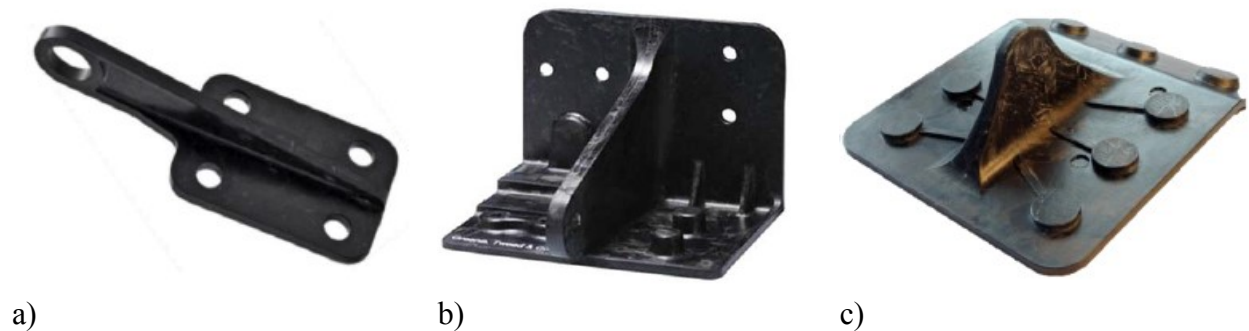
Figure 1-7 – Complex net-moulded industrial ROS parts: a) hinge made by Eguemann [8], b) bracket made by Greene, Tweed [15, 25] and c) bracket made by TenCate [26]
