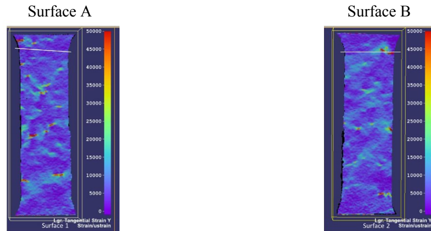
Figure 2-7 – Strain field on the two surfaces of a DCFT specimen visualized with DIC [36]
