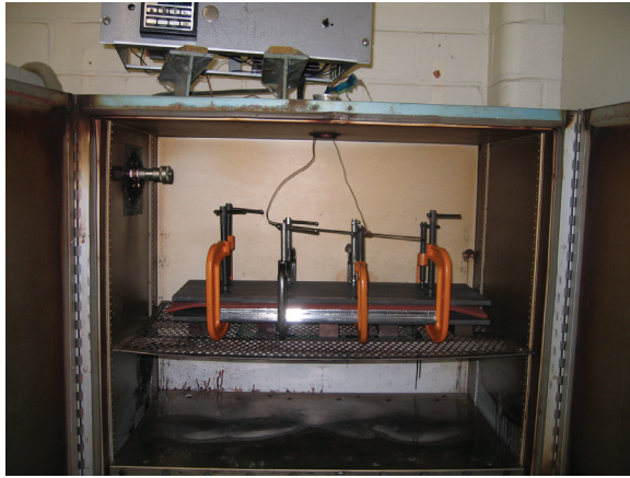
Figure 3.12: METPORE-foam-aluminum-base-plate combination within an oven prior to the start of the heating cycle for curing the epoxy
