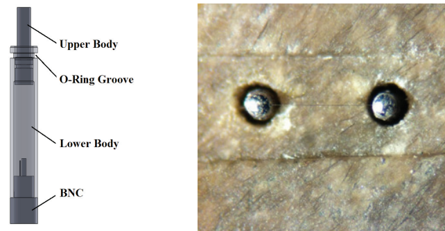
Figure 3.22: Schematic of redesigned sensor (left) and photograph of the hot-wire (right)
