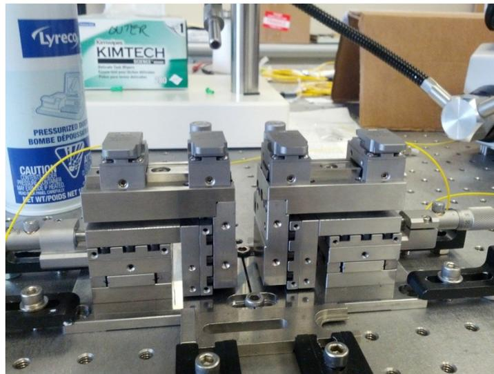
**Figure 4.3: Pigtails placed on XYZ translation stages**
