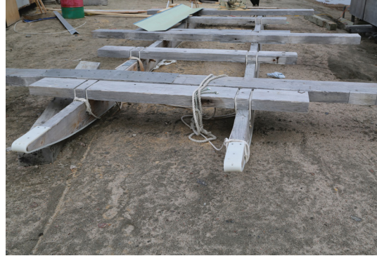
Figure 142. Preparing a made to measure qamutiig for hauling a cabin.
