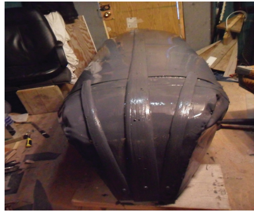
Figure 186. Underside of Isaac's new boat. The plastic water container is waterproofed (Tassugat, 2016).
