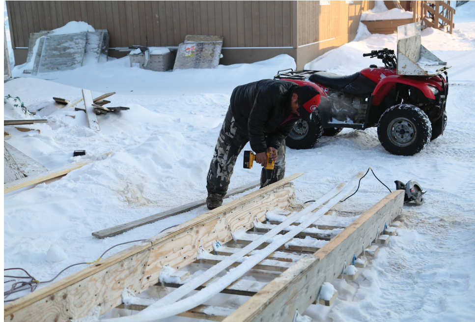
Figure 147. Teflon guards that replace mud guards on qamutiigs.
