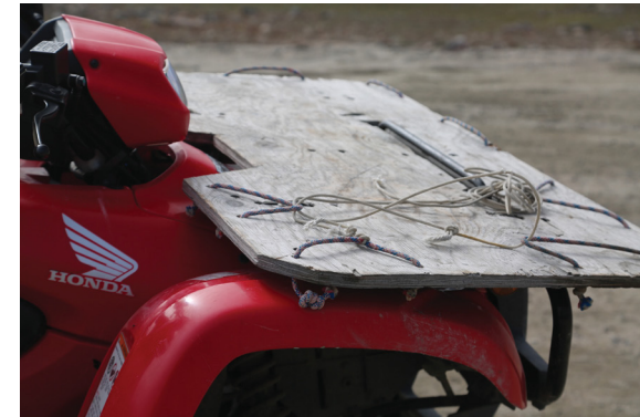
Figure 190. Cargo tray added to the back of an ATV with plywood cut-out.
