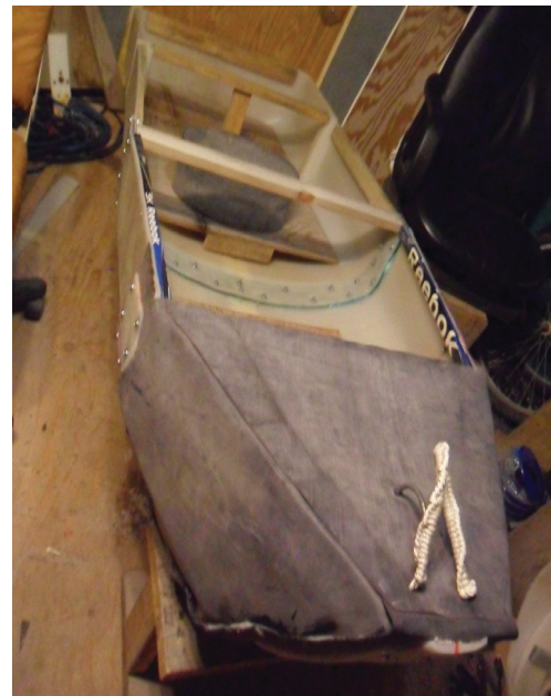
Figure 188. Boat fabricated inside a workshop (Tassugat, 2016). Hockey sticks used as edge reinforcement.
