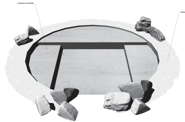
Figure 35. Traditional qarmat foundation, a site found in Clyde River (Havelka, Giraldeau, 2016).
