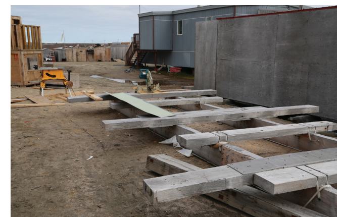
Figure 139. Qamutiiq made to measure prepared to haul a cabin.
