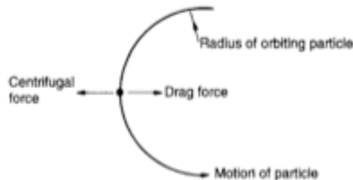
Figure 4: Forces acting on an orbiting particle in the hydrocyclone (Wills and Napier-Munn, 2006)
