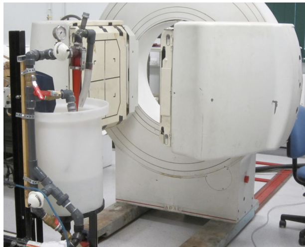
Figure 33: Overview of testing setup with PEPT camera
