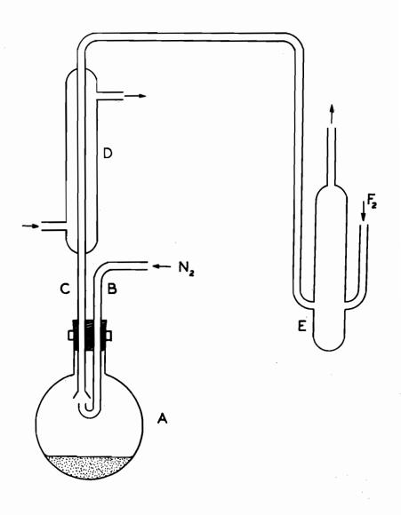
at B. The nitrogen inlet was curved upward into a small flange on the end of the outlet tube. The smoke passed through a water jacket (D) which condensed any sulphur vapor carried through by the nitrogen. It was then led into the reaction tube E, and allowed to react with fluorine which entered at another inlet. The products were condensed in glass traps immersed in liquid air.
