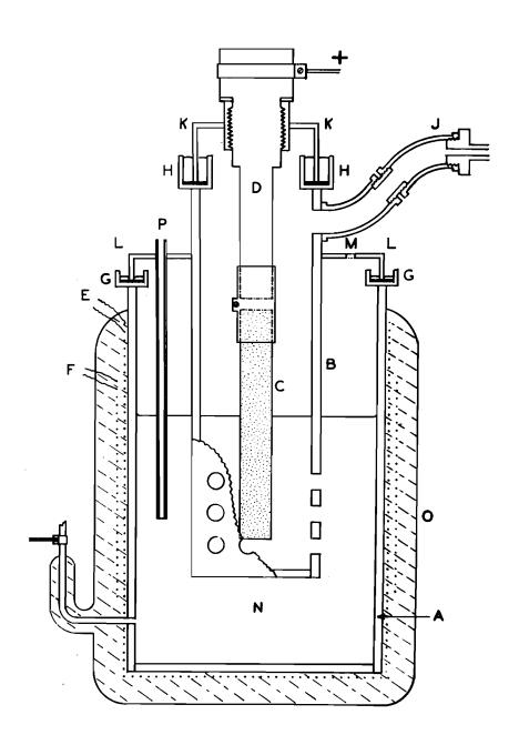
of 1/4" wall thickness and with a welded copper bottom of the same thickness. To allow for diffusion of the electrolyte, three rows of 5/8" holes were drilled around the bottom of the diaphragm.
