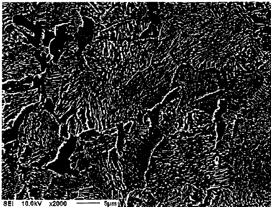
Figure 4.7 As-rolled microstructure of Heat 4.
