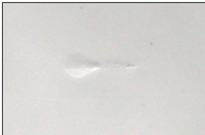
Figure 1. Gas check defect on a PVC film.
