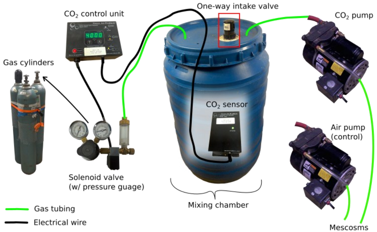
Figure A1.1: Picture diagram illustrating the method for controlling CO 2 in mesocosms. Not pictured: timer controlling pumps, set to ON every sixth fifteen-minute interval (i.e. bubbling for 15 minutes every 1.5 hours). Furthermore, two solenoid valves were used for redundancy.
