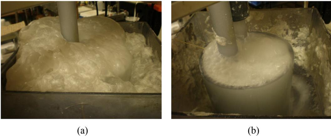
**Fig. 4.17.** In presence of 0.4 M NaCl: (a) Froth build-up in launder after the addition of 1 % w/w talc; (b) Froth collapse after subsequent solvent addition
