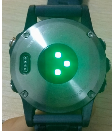
Figure 2.7: A heart rate sensor in working condition on a smart watch.
