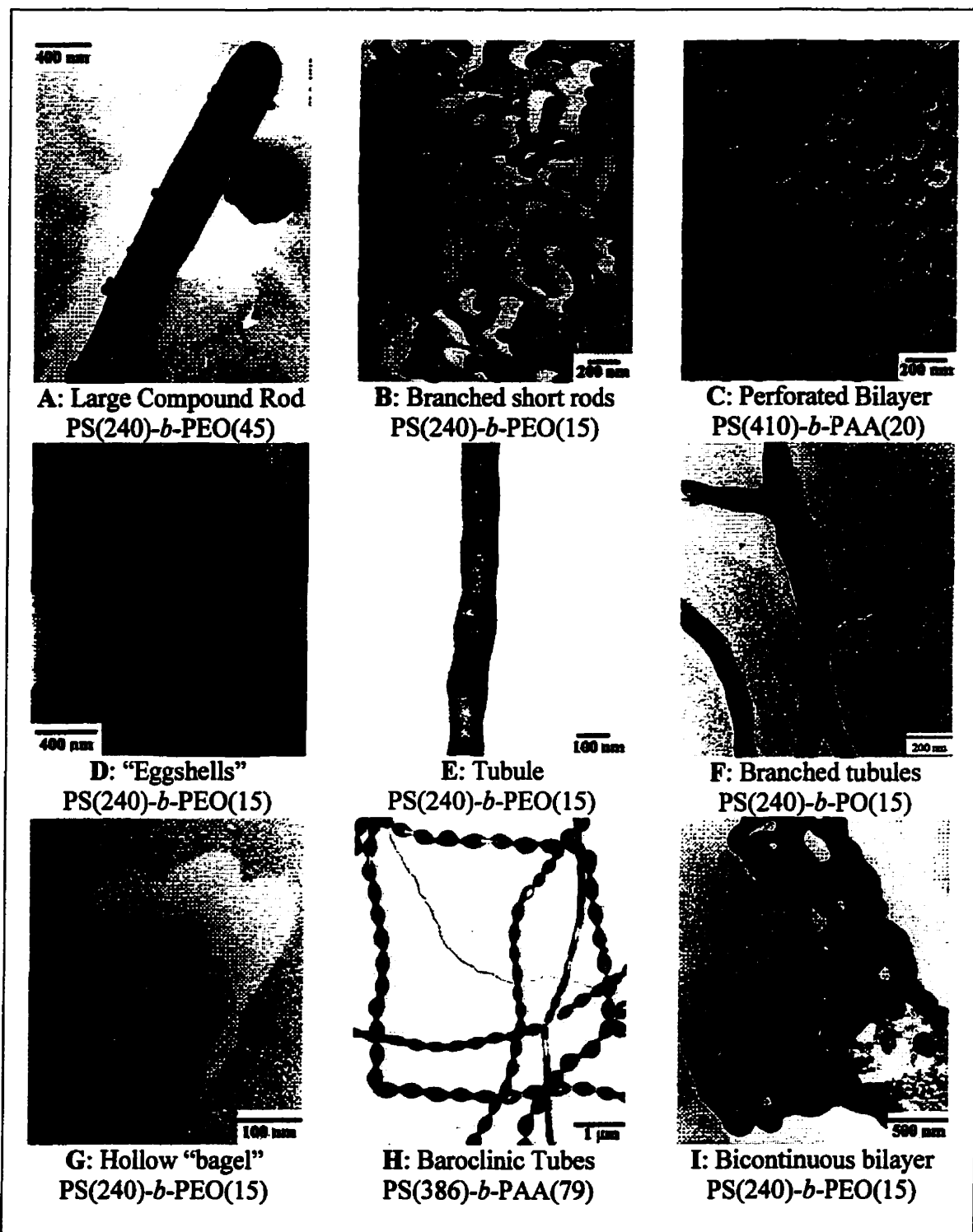
Figure 5: Near-equilibrium morphologies of asymmetric block copolymers in solution.
