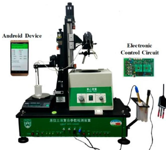
Figure 2-13. Benchtop *in-situ* soil nitrate analyzer using ISEs with soil extraction system. Adapted from Li et al. (2019)
