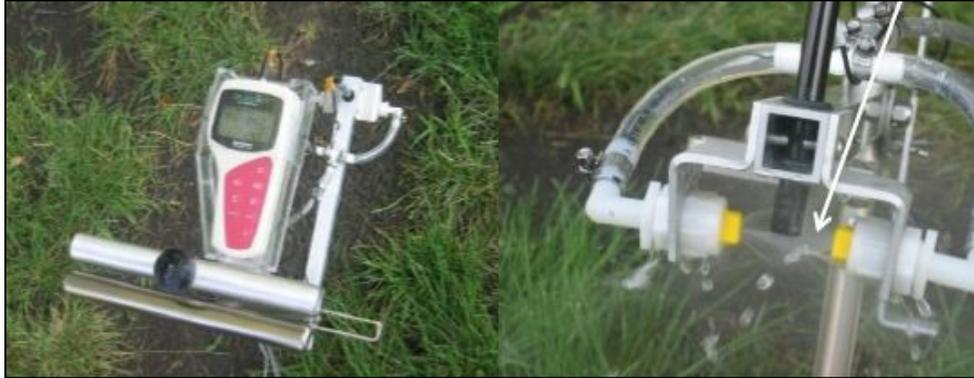
Figure 2-15. Manual probe for on-the-spot soil measurement.
