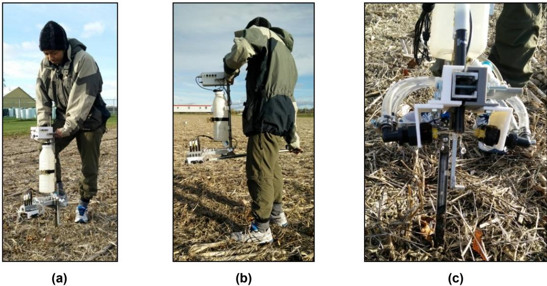
Figure 4-3. Multiple ISEs manual probe operation.
