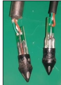
Figure 5-9. Existing Spectrum EC sensor tip
