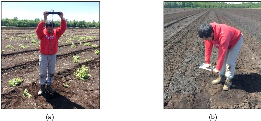
Figure 5-10. Operation of the subsoil manual EC<sub>a</sub> probe: (a) beginning of measurement at the soil surface, (b) end of measurement at 150 cm
