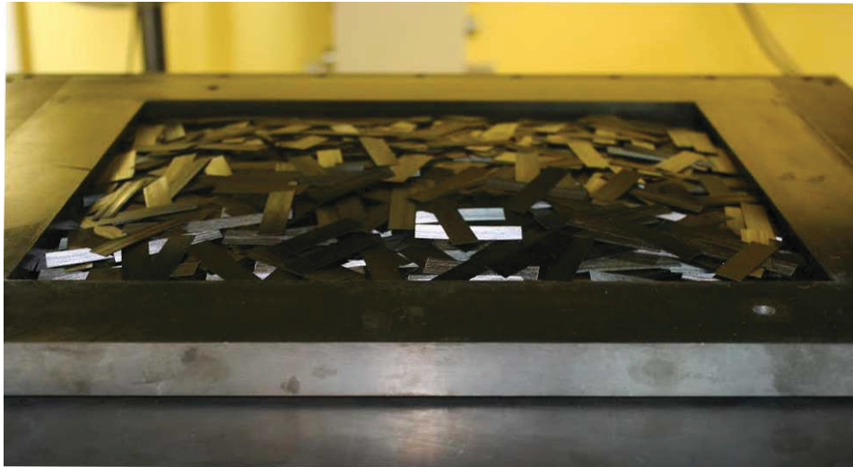
Figure 3.5 – Large flat panel moulding setup showing the DLF strands placed in the mould cavity before processing.
