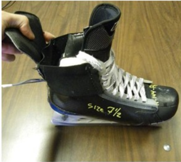
Figure 6: Picture of modified skate with elastic achilles guard
