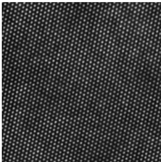
FIGURE 1–3: High resolution TEM image of Si in [110] orientation, demonstrating the effect on phase contrast imaging.
