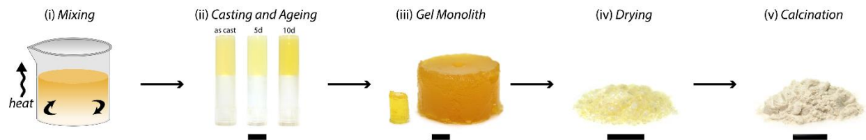
Figure 4.1. An overview of the sol-gel process; (i) mixing of precursor materials, (ii) casting and ageing, (iii) gel monoliths at day 10, (iv) drying, and (v) post calcination at 400 °C (scale bars = 1 cm). (iii) Demonstrates the scaling up possibilities.
