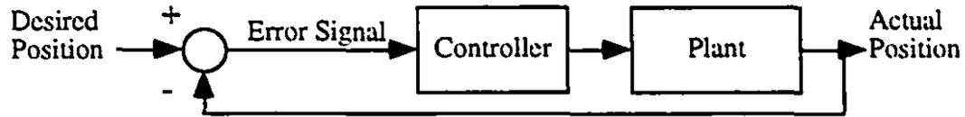
Figure 3.1: Basic control loop for active alignment.
