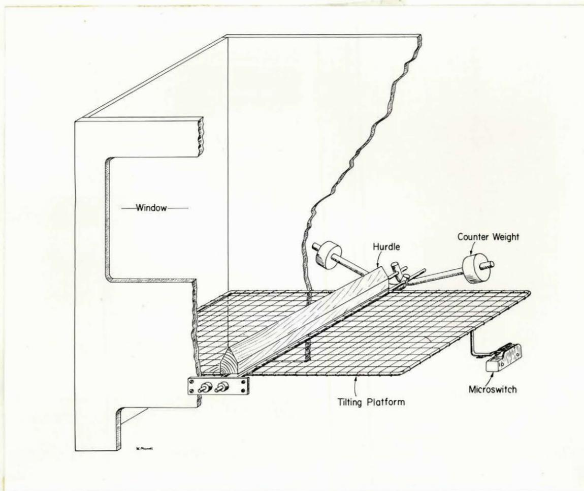
Fig. 1. Diagrammatic representation of the apparatus. Dimensions of the wooden box were 14 x 16 x 10 in. Those of the plexiglass window were  $7\frac{1}{2}$  x 15 in.
