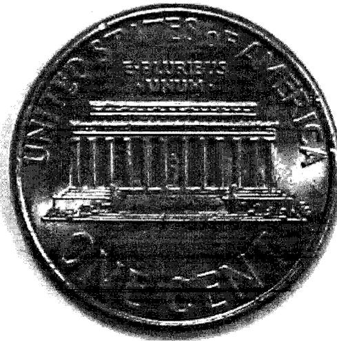
**Figure 4.22** American one cent coin used for imaging experiments. The tail side had its figures but the head side was polished to be flat.
