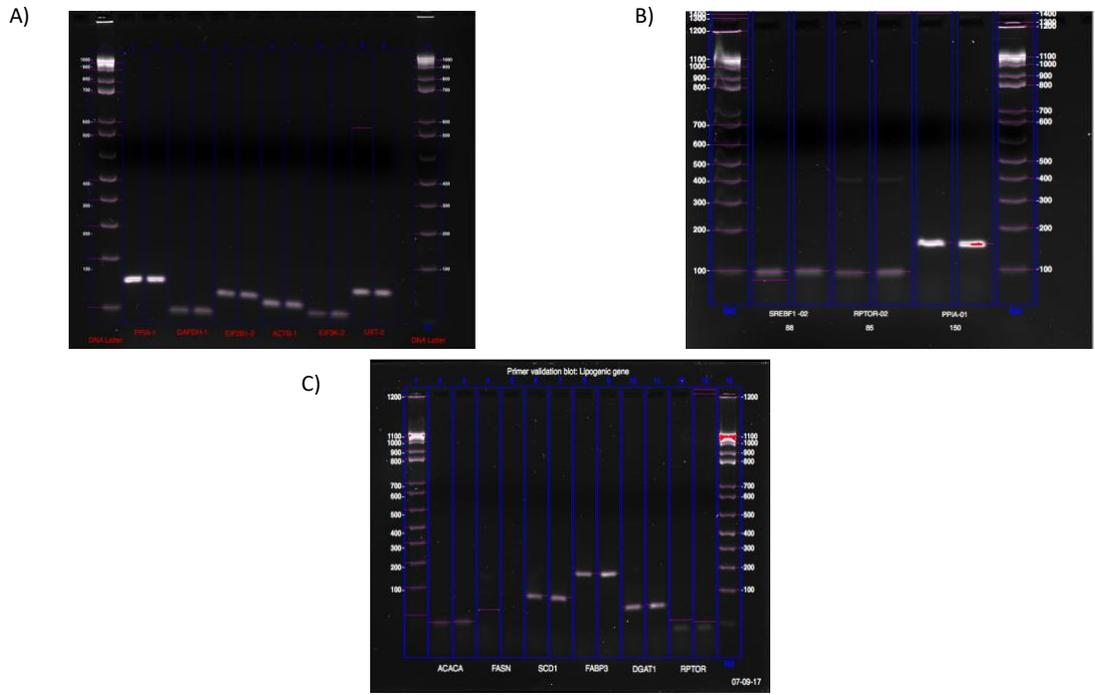
**Figure 3.2: RT-qPCR Validation Information.** Amplicon length was measure for each primer used during experiments. Amplicon length of reference genes: *PPIA*, *GAPDH*, *EIF2B1*, *ACTB*, *EIF3K*, *UXT* (A), target genes: *SREBP1*, *RPTOR*, *PPIA* (B) and lipogenic genes *ACACA*, *FASN*, *SCD1*, *FABP3*, *DGAT1*, *RPTOR2* (C) were measure using ChemiDoc™ imaging system.
