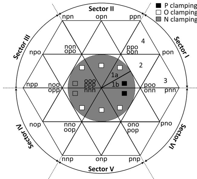
Figure 4-2. Three-level space-vector hexagon with A-phase clamping possibilities; shaded region is for modulation index  $\leq 0.5$
