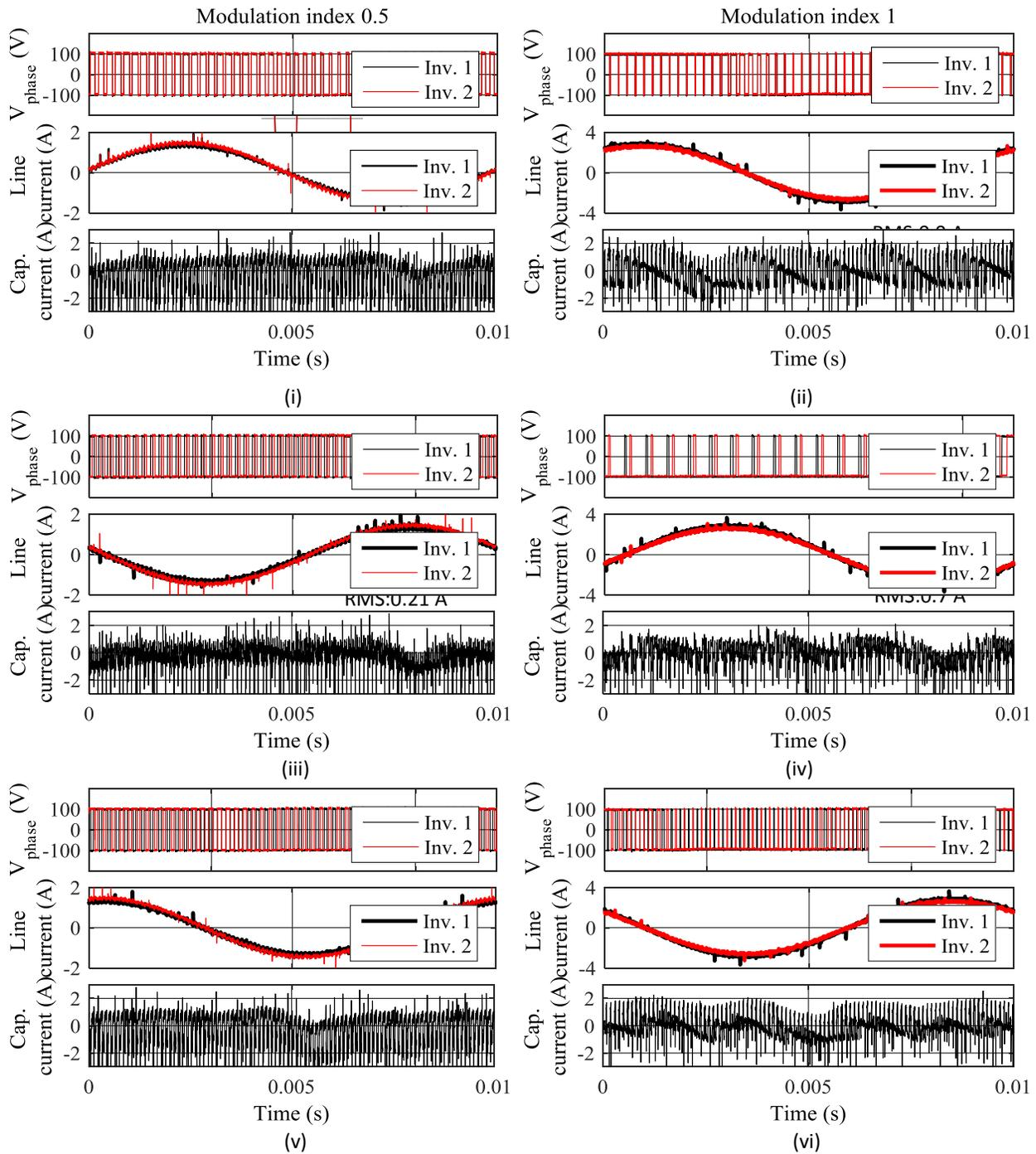
Figure 2-9. Experimental phase voltage (also showing phase difference between pulses of two inverters), Line currents and DC-link capacitor currents for SVPWM with  $0^\circ$  interleaving angle with modulation index (i) 0.5 and (ii) 1; SVPWM with  $90^\circ$  interleaving angle with modulation index (i) 0.5 and (ii) 1; SVPWM with  $180^\circ$  interleaving angle with modulation index (i) 0.5 and (ii) 1
