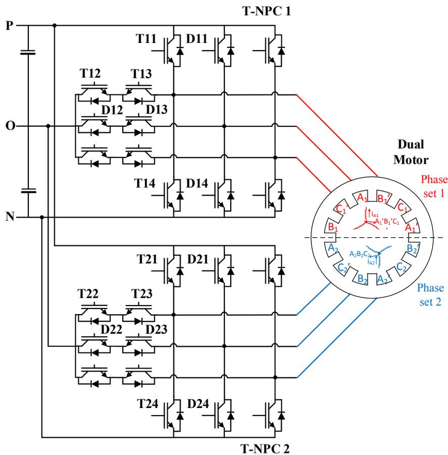
Figure 3-1. Dual T-NPC inverter fed dual PMSM topology
