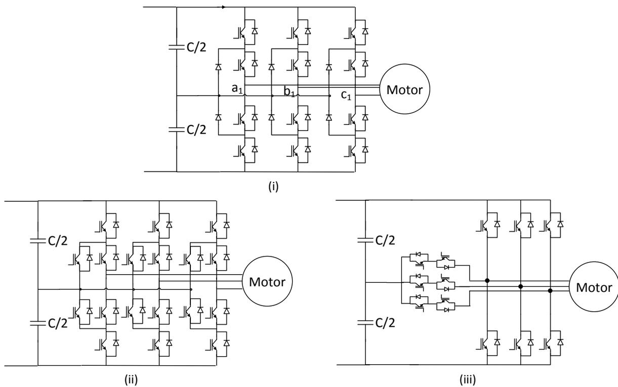
Figure 1-4: (i) NPC inverter (ii) A-NPC inverter (iii) T-NPC Inverter
