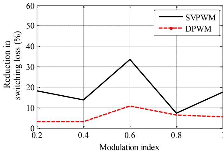
Figure 6-10. Comparison of reduction in switching losses with SVPWM, and DPWM2 operating with variable switching frequency. For DPWM1 and DPWM2 techniques, the values signify switching loss reduction due to variable switching frequency only
