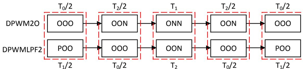
Figure 5-6. Implementation technique of two DPWM strategies (DPWM2O and DPWMLPF2) in sector I, subsector 1b. It also contains the strategy of reduced switching during transition. The rectangles with red dashes show the only allowable transitions between two templates.  $T_1$  is the timing durations of POO or ONN,  $T_2$  is the timing duration of OON, and  $T_0$  is the timing duration of OOO.
