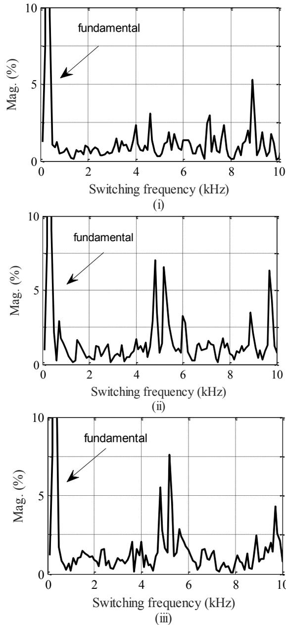
Figure 4-20. Experimental results showing current harmonics for – (i) SVPWM, (ii) *DPWM2O*, and (iii) *DPWM2PN*.
