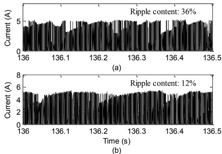
Figure 3-19. Experimental DC-bus current (output current of a single inverter : 5A) - (a) Single T-NPC inverter fed PMSM (b) Dual T-NPC inverter fed dual PMSM
