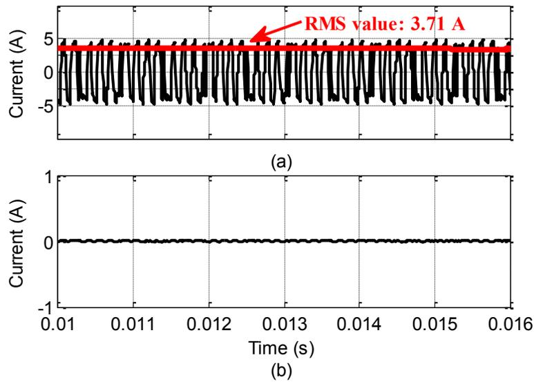
Figure 3-10. DC-link neutral current (a) Single T-NPC inverter fed PMSM (b) Dual T-NPC inverter fed dual PMSM
