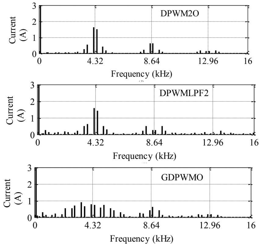
Figure 5-11. Simulation results showing harmonic spectra of line currents at 0.4 modulation index, 0.707 power factor, 120 Hz fundamental frequency and 4.32 kHz switching frequency for –DPWM2O, DPWMLPF2, and GDPWMO.
