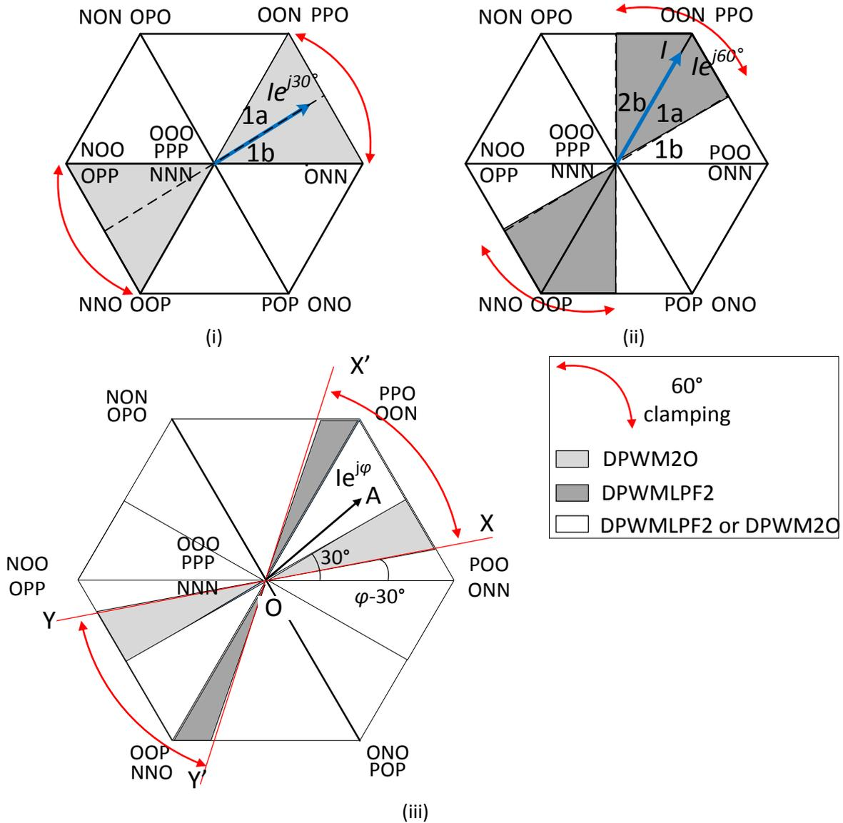
Figure 5-4. The position of the current vector and the clamping strategy with (i) conventional DPWM20, operating with a  $30^\circ$  power factor angle load, (ii) proposed *DPWMLPF2*, operating with a  $60^\circ$  power factor angle load, and (iii) *GDPWMO*, operating with  $\phi$  power factor angle ( $30^\circ \leq \phi \leq 60^\circ$ ) load and combining between *DPWMLPF2* and DPWM20. The intervals shown using the red colored arrows are the  $60^\circ$  clamping durations
