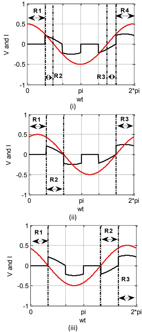
Figure Ap\_A-4: Modulation voltage waveform and current waveform for DPWM20 with (i)  $0^\circ$ , (ii)  $30^\circ$  and (iii)  $-30^\circ$  power factor angle
