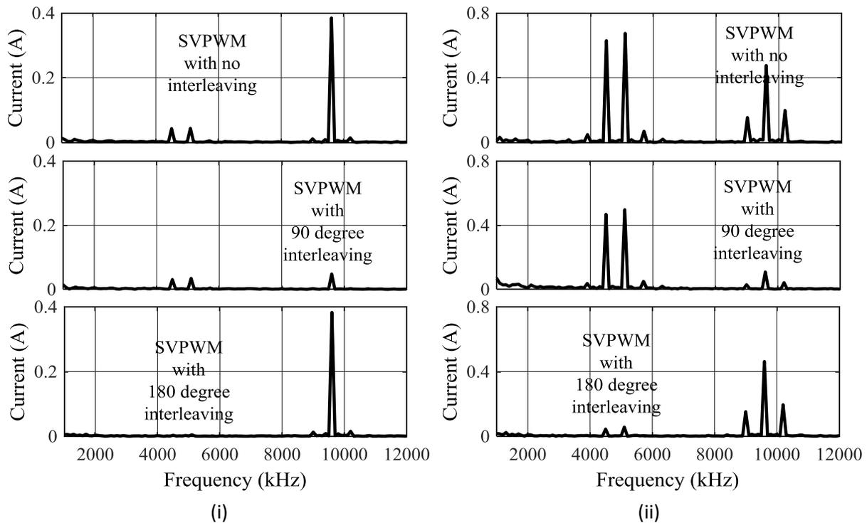
Figure 2-10. Experimental results - Capacitor harmonic spectrum for (i)  $m: 0.5$ , SVPWM with  $0^\circ$ ,  $90^\circ$  and  $180^\circ$  interleaving angle (top to bottom) and (ii)  $m: 1$ , SVPWM with  $0^\circ$ ,  $90^\circ$  and  $180^\circ$  interleaving angle (top to bottom)
