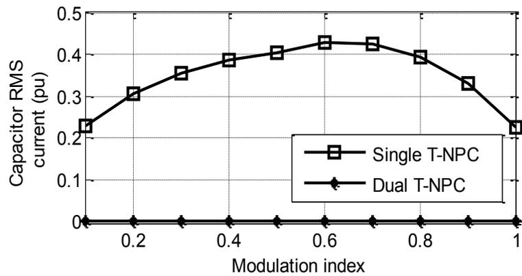
Figure 3-11. Difference in DC-link capacitor RMS current
