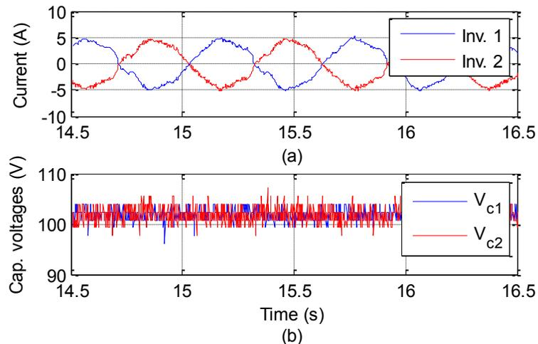
Figure 3-16. Experimental results of dual T-NPC inverter fed dual PMSM ( $V_{dc}$ : 200 V, o/p current: 5A) - (a) line currents (b) capacitor voltages
