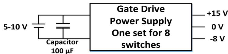
Figure Ap\_B-2: Gate drive Power supply block diagram for 8 switches with DC power supply and bypass capacitor; three such sets in the setup
