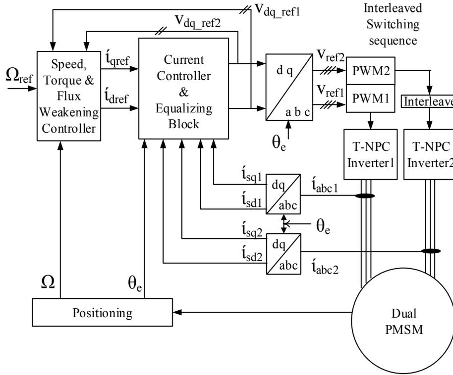
Figure 3-4. Overall control strategy of the dual inverter system
