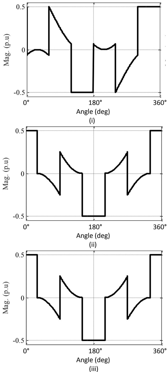
Figure 4-4. Average phase to DC-link neutral voltage waveforms for modulation index less than 0.5, normalized w.r.t DC-link voltage - (i) *DPWM0PN*; (vi) *DPWM1PN*; (vii) *DPWM2PN*
