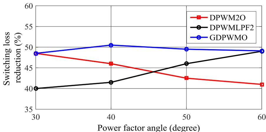
Figure 5-12. Comparisons of switching loss reduction using DPWM2O, DPWMLPF2 and GDPWMO sequences for different operating power factor
