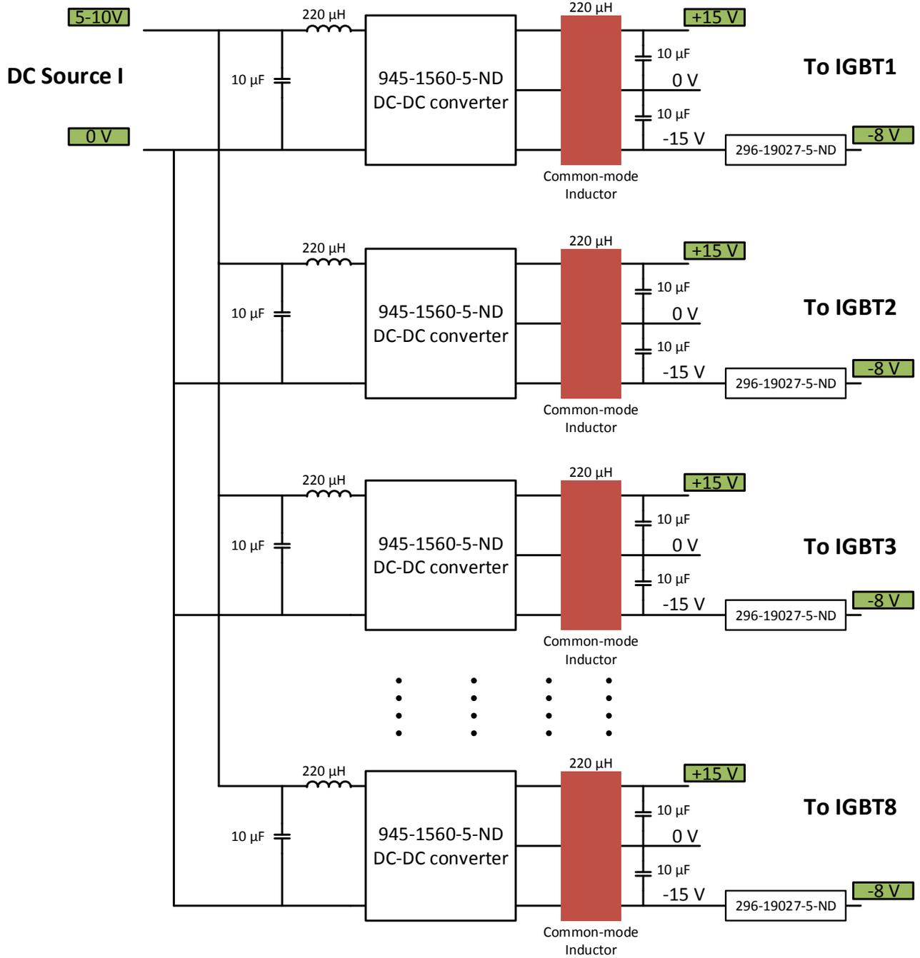
Figure Ap\_B-3: Circuit diagram and components of Gate drive power supply (for 8 switches)
