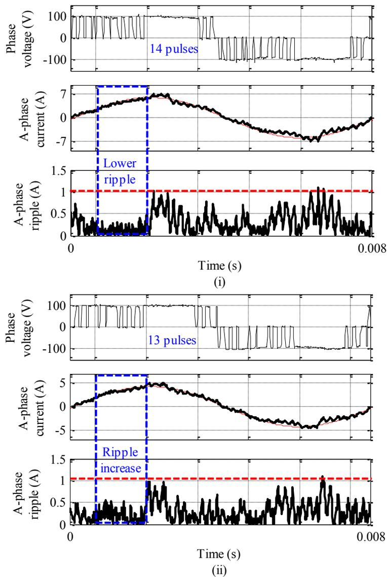
Figure 6-15. Comparison of experimental phase voltage, number of switching, current, and current ripple for DPWM with (i) constant and (ii) variable switching frequency, Operating modulation index=0.95
