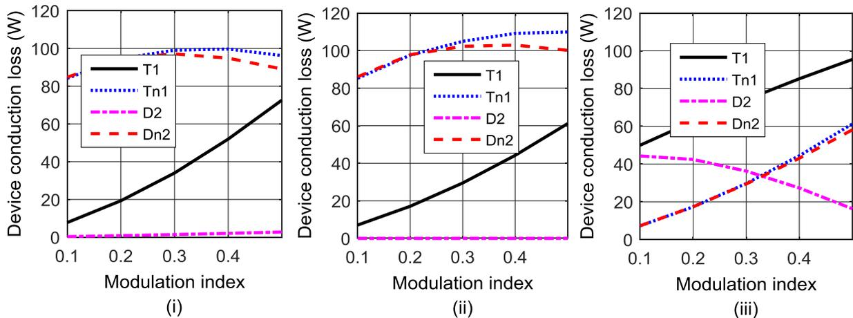
Figure 4-12. Simulation results showing conduction loss distribution amongst different switching devices for – (i) SVPWM, (ii) DPWM2O, and (iii) DPWM2PN.
