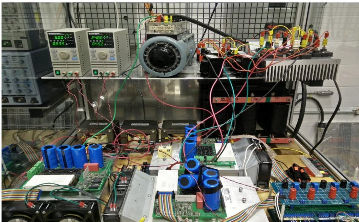
Figure 2-7. Experimental setup of Dual two-level inverter
