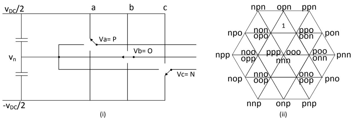
Figure 1-5: (i) Three-level Inverter operation, (ii) Three-level Inverter switching vectors
