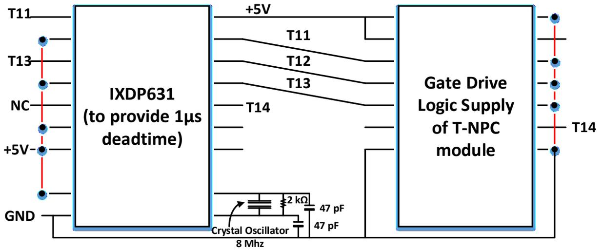
Figure Ap\_B-4: Circuit diagram and components of Gate drive logic supply (for 4 switches in one leg)
