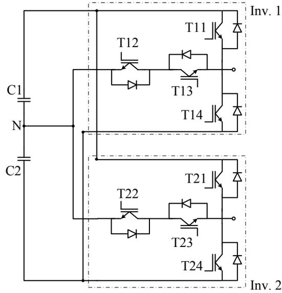
Figure 3-3. A single leg of T-NPC inverter
