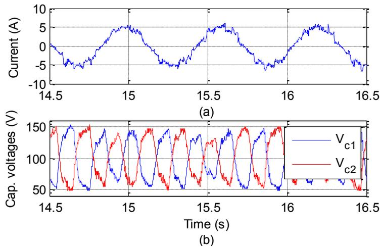
Figure 3-15. Experimental results of single T-NPC inverter fed PMSM ( $V_{dc}$ : 200 V, output current: 5A) - (a) line current (b) capacitor voltages
