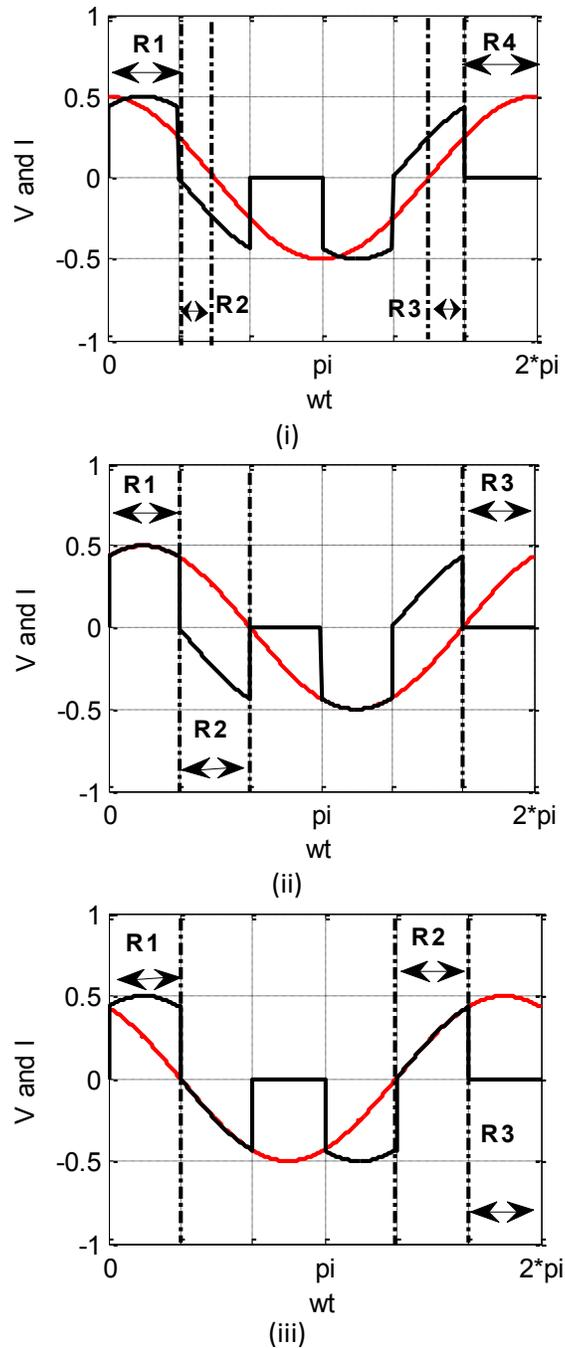
Figure Ap\_A-6: Modulation voltage waveform and current waveform for DPWM00 with (i)  $0^\circ$ , (ii)  $30^\circ$  and (iii)  $-30^\circ$  power factor angle,
