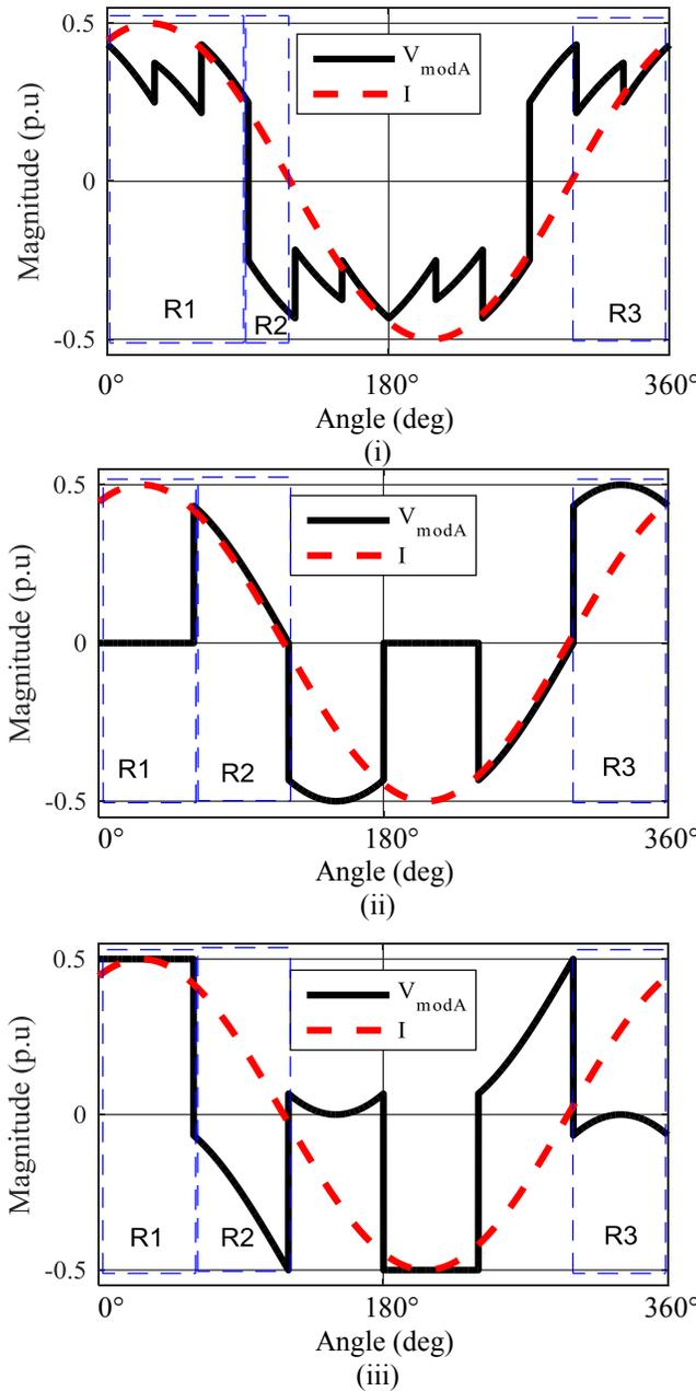
Figure 4-5. Average phase to DC-link neutral voltage waveforms and current waveforms for (i) SVPWM, (ii) DPWM2O, and (iii) DPWM2PN for 30° power factor angle. It shows the regions (R1, R2 and R3) in the positive half-cycle of the current. The regions signify different possibilities of device conducting.
