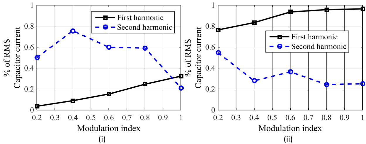
Figure 2-8. Experimental results - first and second switching frequency harmonic components for (i) SVPWM, and (ii) DPWM2 strategies for single inverter
