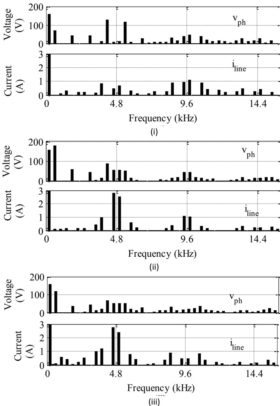
Figure 5-9. Simulation results showing harmonic spectra of phase to DC-link neutral voltage and line currents at 0.4 modulation index, 0.5 power factor, 200 Hz fundamental frequency and 4.8 kHz switching frequency for – (i) SVPWM, (ii) DPWM2O, and (iii) DPWMLPF2.
