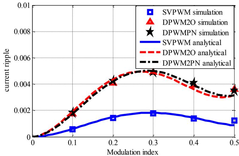
Figure 4-15. Simulated and analytical results of the dependency of the RMS value of output line current ripple on the modulation index
