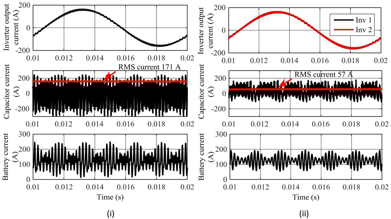
Figure 2-4. Line currents, DC-link capacitor currents, DC-link capacitor RMS current and battery current for (i) without interleaving and (ii) with interleaved SVPWM
