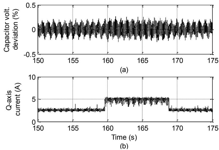
Figure 3-20. Experimental results of transient operation of dual T-NPC inverter fed dual PMSM (a) Capacitor voltage deviation (b) Change in dual motor current (from 2.5 A to 5 A)
