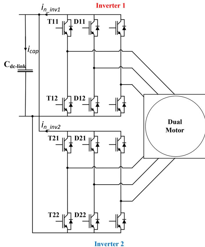
Figure 2-1. Dual 2-level inverter feeding a dual 3-phase PMSM (180° phase-shifted stator winding sets)
