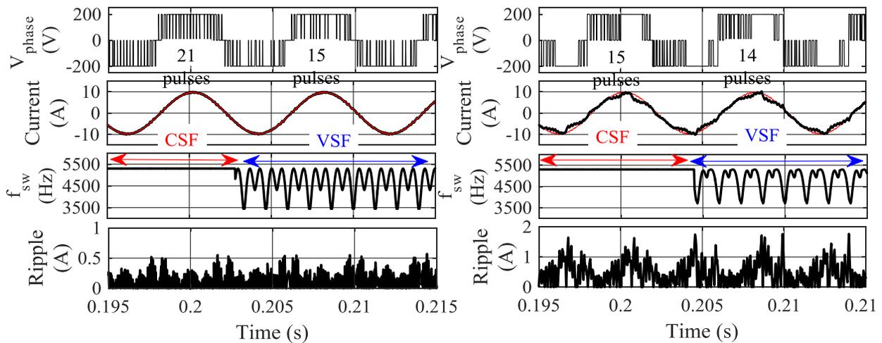
Figure 6-9. Comparison of phase A current, number of switching, current ripple and switching frequency variation for (i) SVPWM, and (ii) DPWM2 at constant and variable switching frequency the SVPWM and DPWM2. The variation in SVPWM is higher than DPWM2 because of a higher current ripple variation in a sector for SVPWM, compared to DPWM2.
