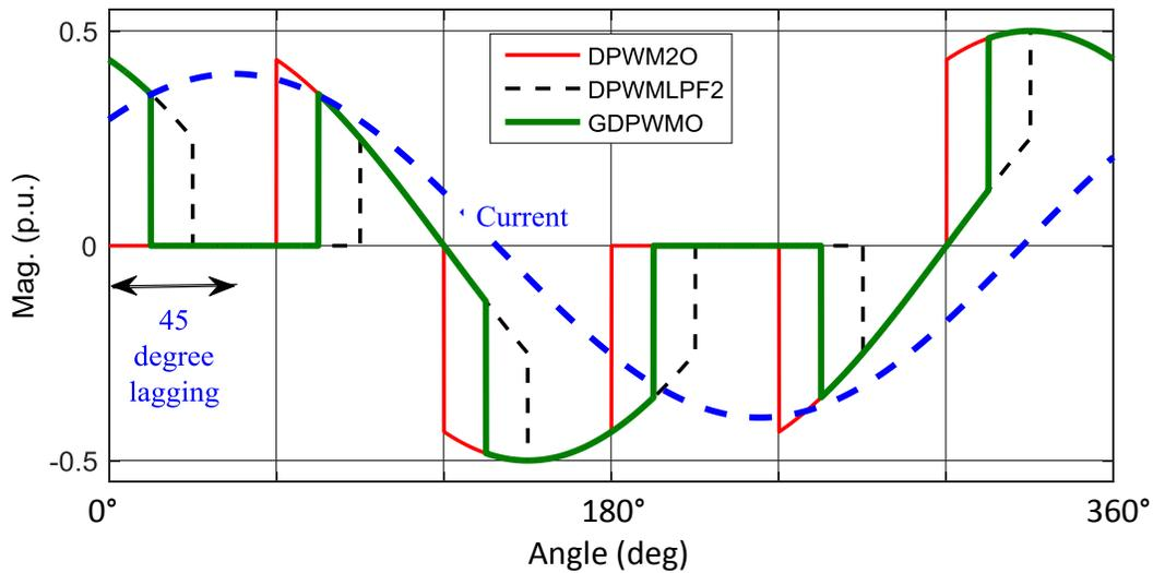
Figure 5-5. Phase difference between a-phase fundamental current (power factor 0.707) and average phase to DC-link neutral voltage waveforms for DPWM2O, DPWMLPF2 and GDPWMO. The peaks of the line current are aligned with GDPWMO
