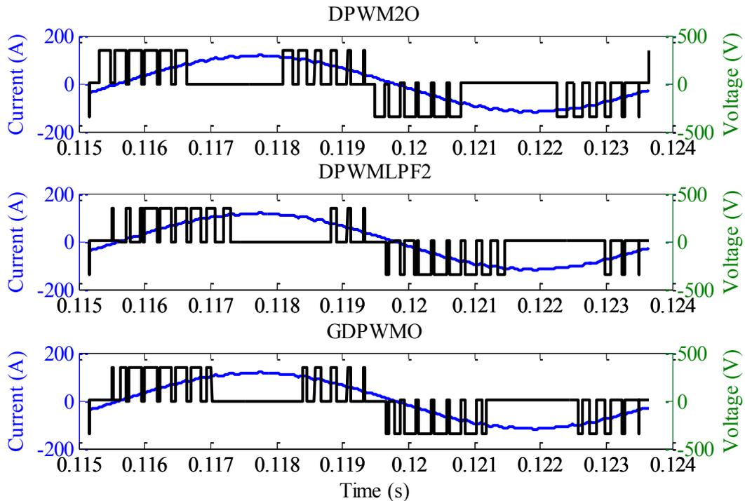
Figure 5-10. Simulation results showing phase to DC-link neutral voltage and line currents at 0.4 modulation index, 0.707 power factor, 120 Hz fundamental frequency and 4.32 kHz switching frequency for – (i) DPWM20, (ii) DPWMLPF2, and (iii) GDPWMO.
