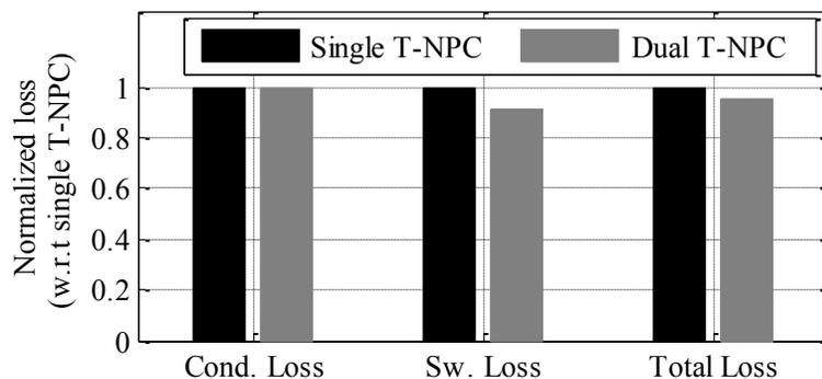
Figure 3-12. Loss reduction using Dual T-NPC topology operating with DPWM techniques
