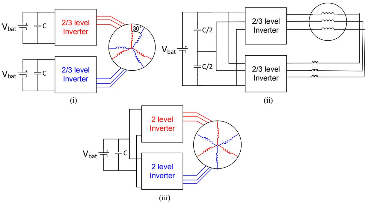
Figure 1-7: Dual Inverter topologies with (i) Dual PMSM ( $30^\circ$  phase shifted) (ii) Open-winding motor (iii) Dual PMSM ( $180^\circ$  phase shifted) motor
