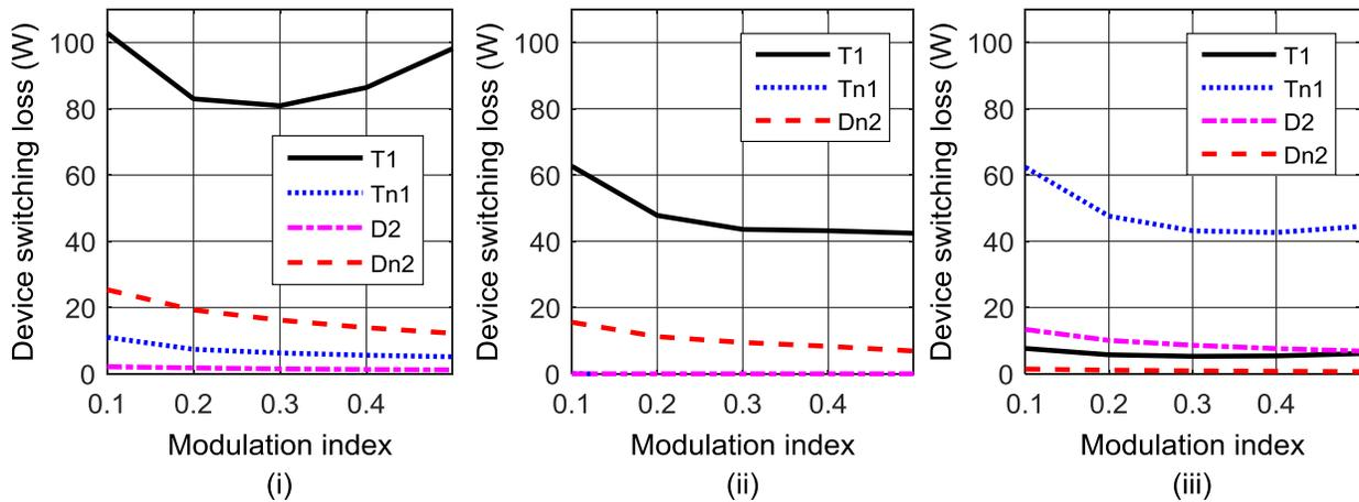
Figure 4-11. Simulation results showing switching loss distribution amongst different switching devices for – (i) SVPWM, (ii) DPWM2O, and (iii) DPWM2PN.
