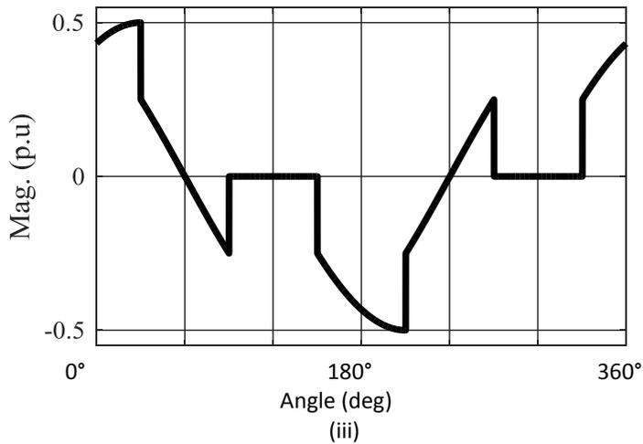
Figure 5-2. Average phase to DC-link neutral voltage [28] waveforms for modulation index less than 0.5, normalized w.r.t DC-link voltage for proposed DPWM templates - (i) *DPWMLPF1*; (ii) *DPWMLPF2*; (iii) *DPWMLPF3* ; 0.5 signifies half DC-link voltage
