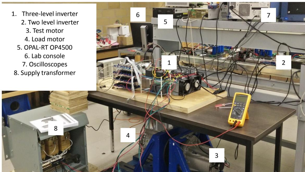
Figure 6-12. Experimental setup of three-level T-type inverter feeding a motor load
