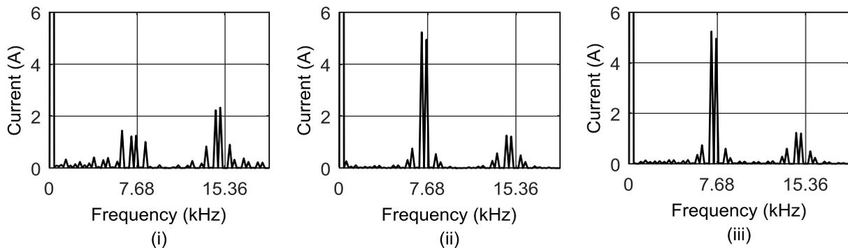
Figure 4-10. Simulation results showing current harmonics for – (i) SVPWM, (ii) DPWM2O, and (iii) DPWM2PN. Fundamental frequency component: 86 A
