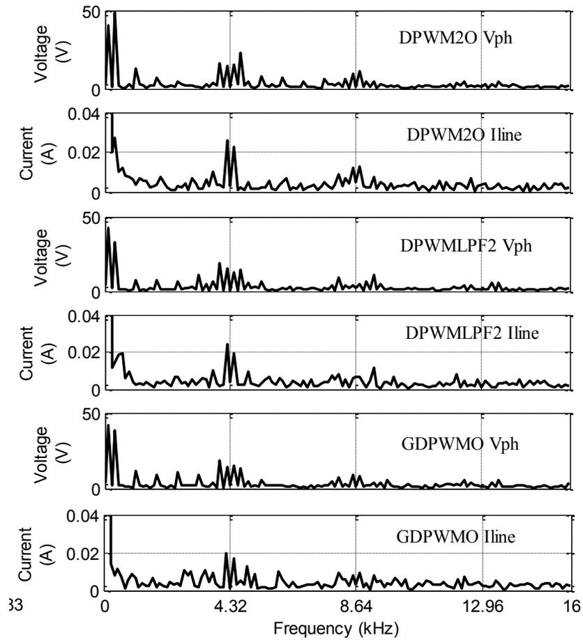
Figure 5-17. Experimental (i) phase-DC-link neutral voltages, line currents, and (ii) their harmonic spectra for DPWM2O, DPWMLPF2 and GDPWMO - experimental conditions (modulation index: 0.4, fundamental frequency: 120 Hz, switching frequency: 4320 Hz, power factor: 0.707, time step: 1 ms/div). Red rectangles show current peaks
