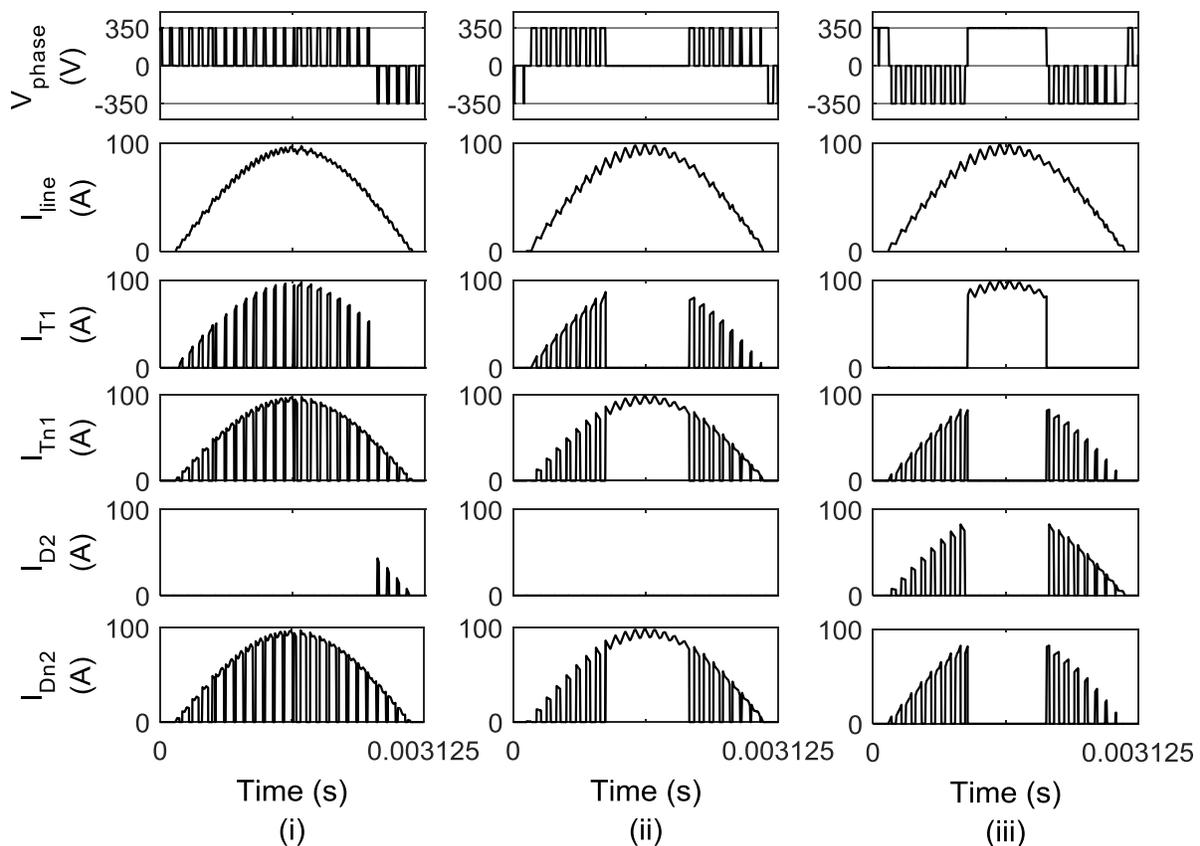
Figure 4-9. Simulation results showing phase to DC-link neutral voltage, line currents,  $T1$  currents,  $Tn1$  currents,  $D2$  currents and  $Dn1$  currents at 0.4 modulation index, 0.866 power factor, 160 Hz fundamental frequency and 7.68 kHz switching frequency for – (i) SVPWM, (ii) DPWM2O, and (iii) DPWM2PN.
