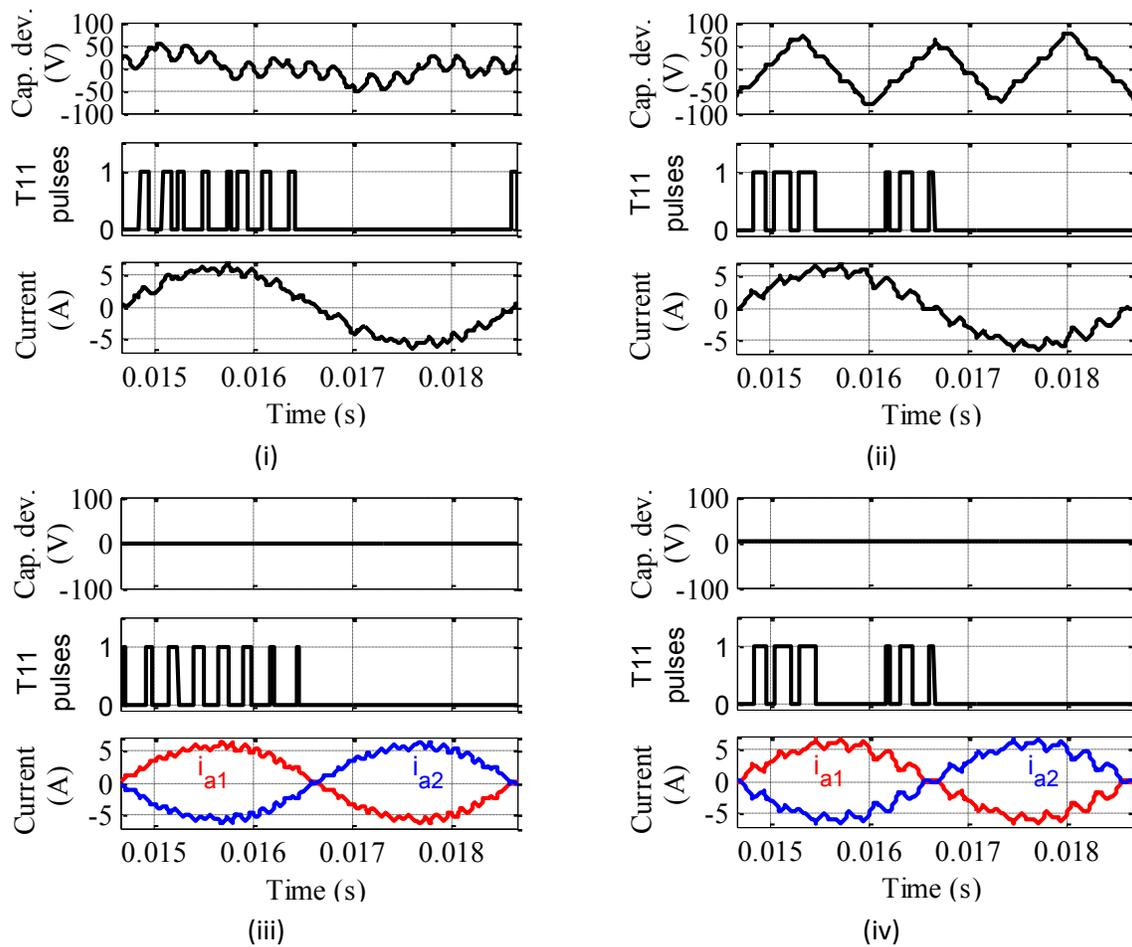
Figure 3-6. Capacitor voltage deviation, number of IGBT pulses and output line currents: (i) Single T-NPC with SVPWM employing passive capacitor voltage balancing, (ii) Single T-NPC with DPWM with no capacitor voltage balancing ability, (iii) Dual T-NPC with SVPWM having no additional switching instances, and (iv) Dual T-NPC with DPWM with no capacitor voltage balancing ability.
