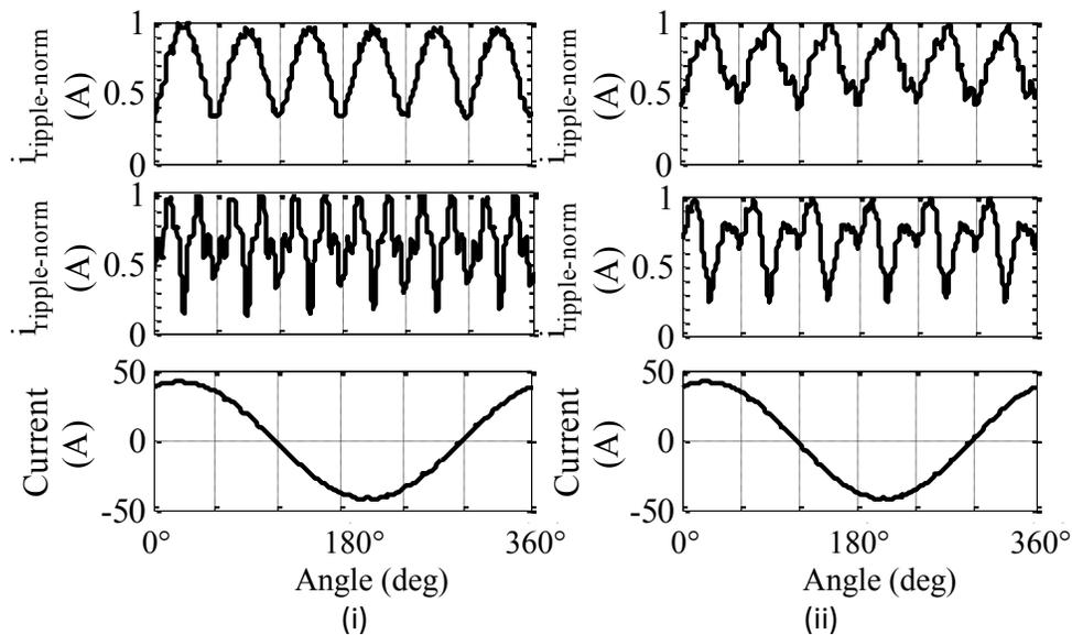
Figure 6-8. Current ripple variation comparison of (i) SVPWM, and (ii) DPWM2
