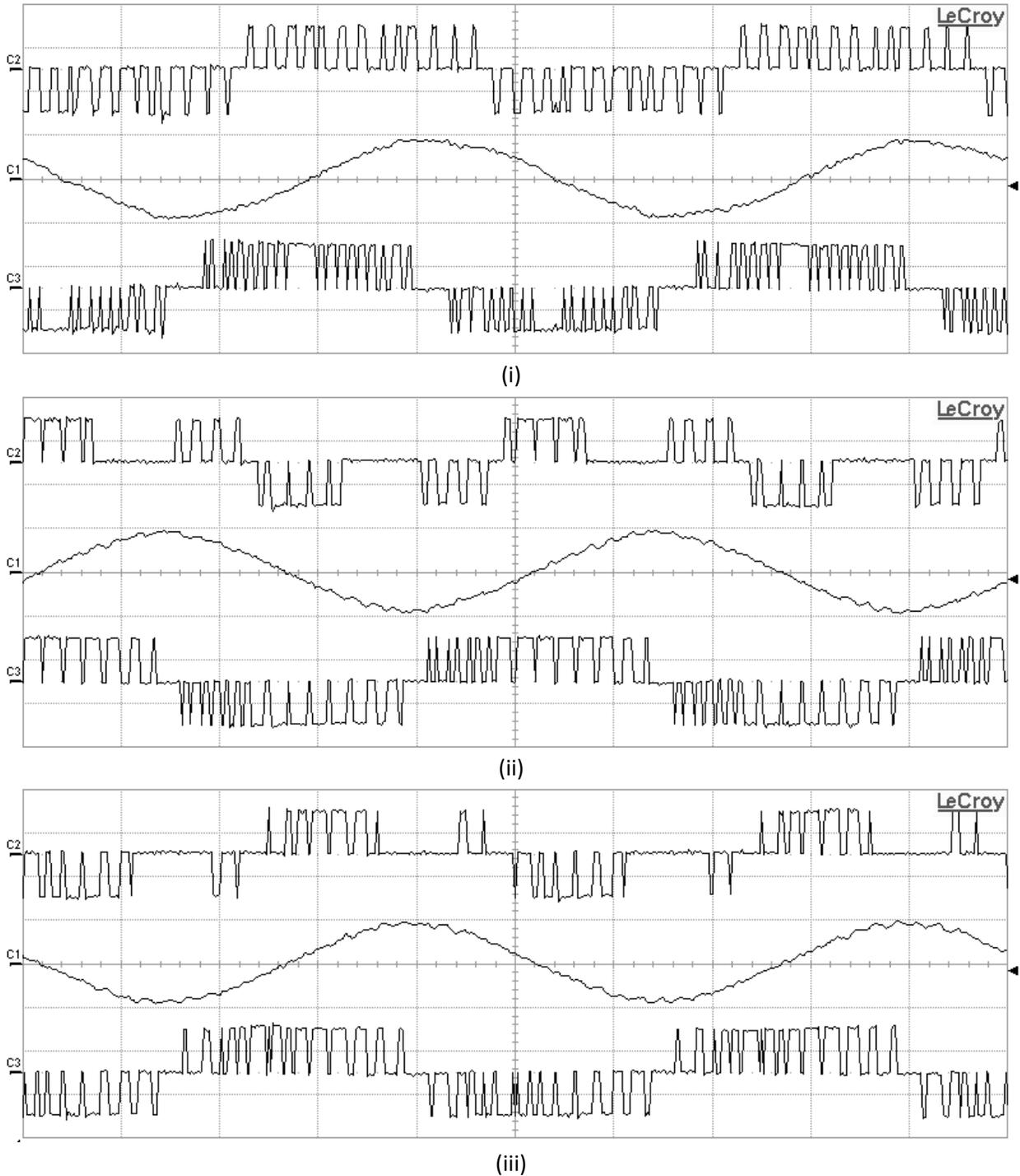
Figure 5-13. Experimental phase-DC-link neutral voltages ( $V_{ph} : 100 \text{ V/div}$ ) and line currents ( $I_{line}: 2 \text{ A/div}$ ) for (i) SVPWM, (ii) DPWM2O, and (iii) DPWMLPF - experimental conditions (modulation index: 0.4, fundamental frequency: 200 Hz, switching frequency: 4800 Hz, power factor: 0.5, time step: 1 ms/div).
