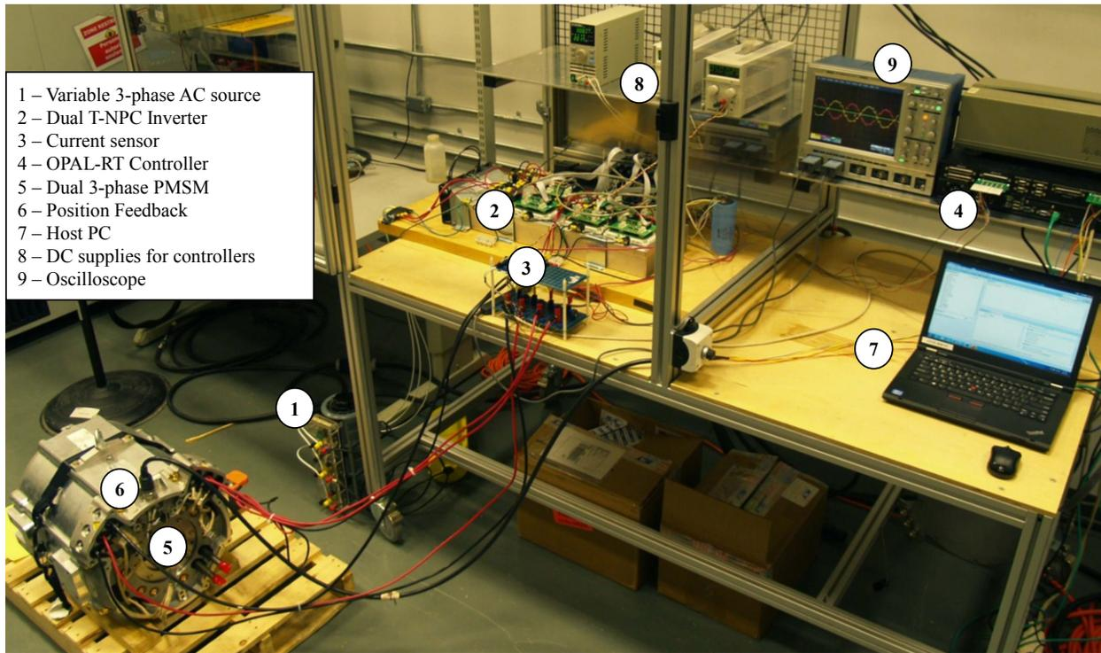
Figure 3-14. Experimental setup of the dual three-level T-NPC inverter fed dual PMSM topology
