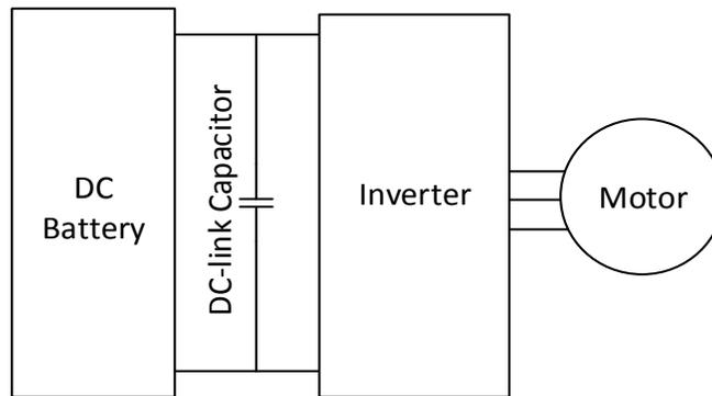
Figure 1-1: A generic diagram showing Inverter fed Motor drive from a DC battery
