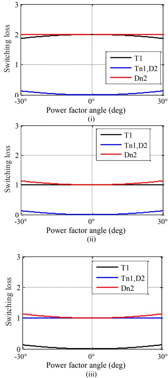
Figure 4-6. Device switching loss comparison between (i) SVPWM, (ii) DPWM2O, and (iii) DPWM2PN over change in power factor angle
