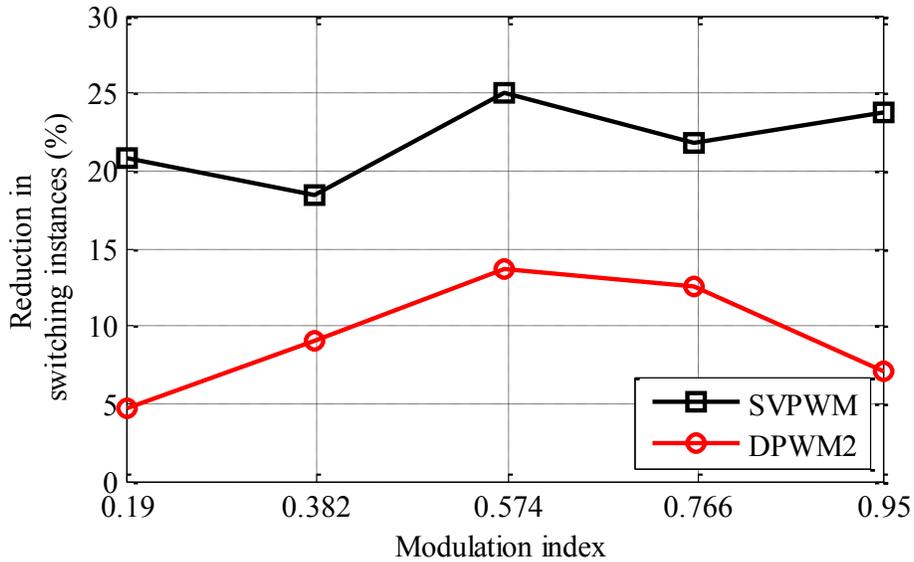
Figure 6-16. Comparison of reduction in switching losses with SVPWM, and DPWM2 operating with variable switching frequency. For DPWM1 and DPWM2 techniques, the values signify switching loss reduction due to variable switching frequency only
