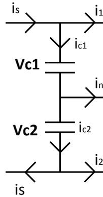
Figure Ap\_A-3: Three-level dc-link capacitor current and voltages
