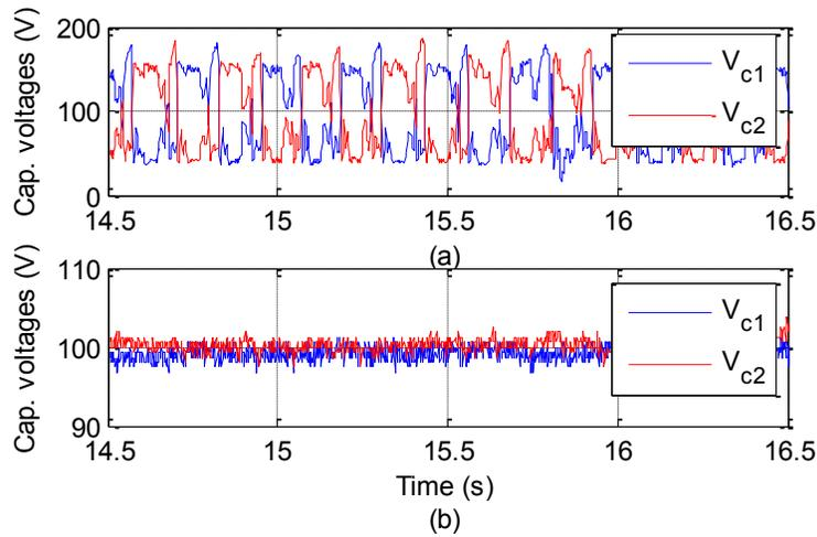
Figure 3-17. Experimental DC-link capacitor voltages with discontinuous PWM strategy ( $V_{dc}$ : 200 V, output current of a single inverter: 5A) - (a) Single T-NPC inverter fed PMSM (b) Dual T-NPC inverter fed dual PMSM
