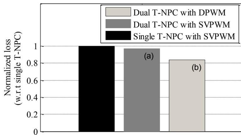
Figure 3-22. Experimental result showing inverter loss reduction using Dual T-NPC topology (output current of a single inverter: 5A, speed of the motor: 240 RPM) - (a) due to absence of additional switching instances of single T-NPC topology and (b) using DPWM technique
