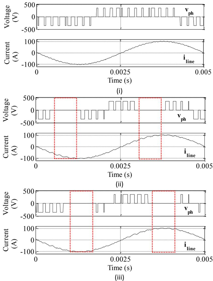
Figure 5-8. Simulation results showing phase to DC-link neutral voltage and line currents at 0.4 modulation index, 0.5 power factor, 200 Hz fundamental frequency and 4.8 kHz switching frequency for – (i) SVPWM, (ii) DPWM2O, and (iii) DPWMLPF2.
