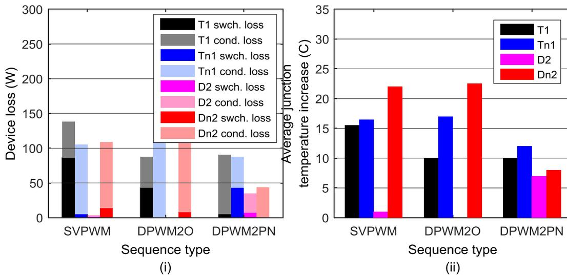
Figure 4-13. Simulation results showing (i) total inverter loss distribution amongst different switching devices, and (ii) device average temperature rise distribution for SVPWM, DPWM2O, and DPWM2PN.
