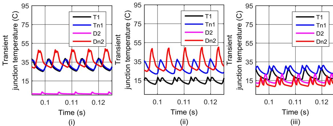
Figure 4-14. Simulation results showing transient junction temperature distribution amongst different switching devices for – (i) SVPWM, (ii) DPWM2O, and (iii) DPWM2PN.
