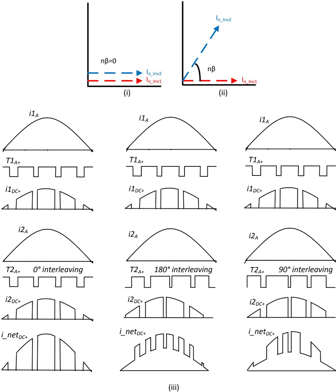
Figure 2-3. Capacitor nth harmonic contents (i) Interleaving angle  $0^\circ$ , (ii) Interleaving angle  $n\beta$ , (iii) graphical waveform showing impact of interleaving on positive DC bus current ripple
