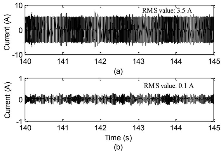
Figure 3-18. Experimental results of DC-link capacitor current dual T-NPC inverter fed dual PMSM ( $V_{dc}$ : 200 V, output current of each inverter: 5A) - (a) Single T-NPC inverter fed PMSM (b) Dual T-NPC inverter fed dual PMSM
