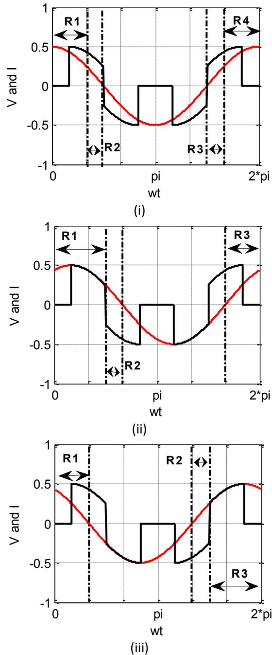
Figure Ap\_A-5: Modulation voltage waveform and current waveform for DPWM10 with (i)  $0^\circ$ , (ii)  $30^\circ$  and (iii)  $-30^\circ$  power factor angle
