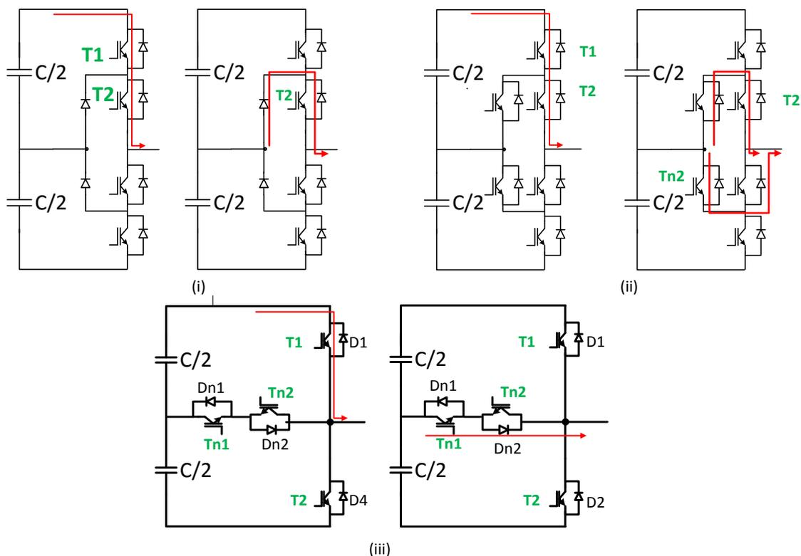
Figure 1-6: Inverter Switching Transitions (P to O) (i) NPC Inverter, (ii) A-NPC Inverter, (iii) T-NPC Inverter
