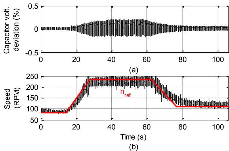
Figure 3-21. Experimental results of transient operation of dual T-NPC inverter fed dual PMSM (a) Change in speed (80 RPM→240 RPM→120 RPM) (b) Capacitor voltage deviation
