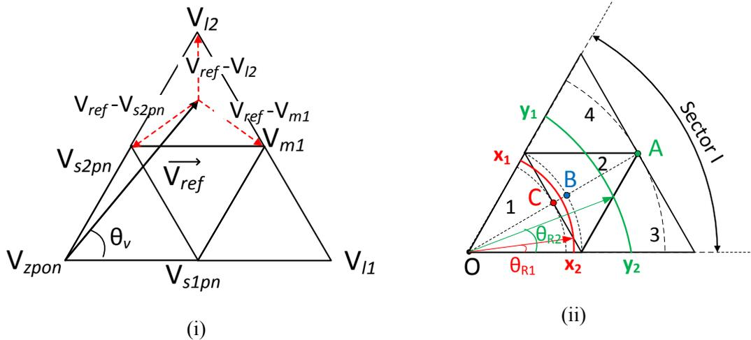
Figure 6-1. (i) Three-level space vector hexagon, switching vectors, sector I and subsector division. Also shows the deviation vectors generated because of discrete switching states of a PWM inverter, (ii) A 60-degree sector (sector I) showing subsectors, operating regions of the voltage vector and its duration of stay in different subsectors.
