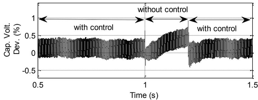
Figure 3-9. Effect of the controller in maintaining balancing
