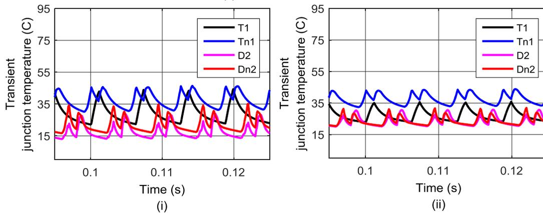
Figure 4-16. Simulation results showing transient junction temperature distribution for DPWM2PN using (i) 30% more current, and (ii) 37.5% higher switching frequency
