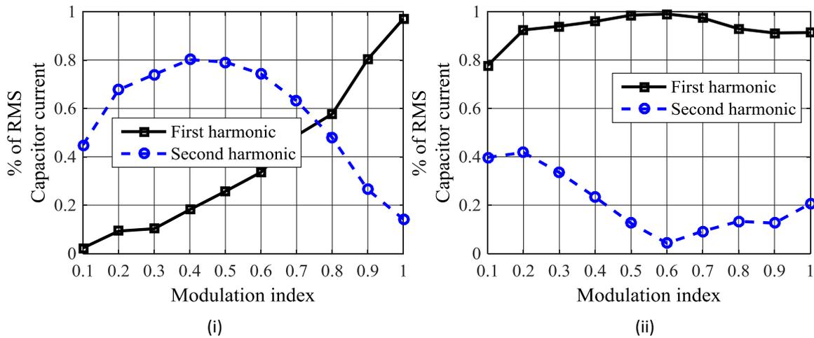
Figure 2-2. First and Second switching frequency harmonic components for (i) SVPWM, and (ii) DPWM2 strategies for single inverter frequency harmonic components for (i) SVPWM, and (ii) DPWM2 strategies for single inverter
