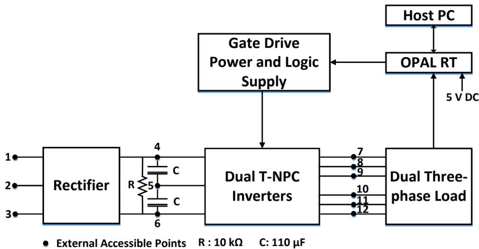
Figure Ap\_B-1: Experimental Setup schematics
