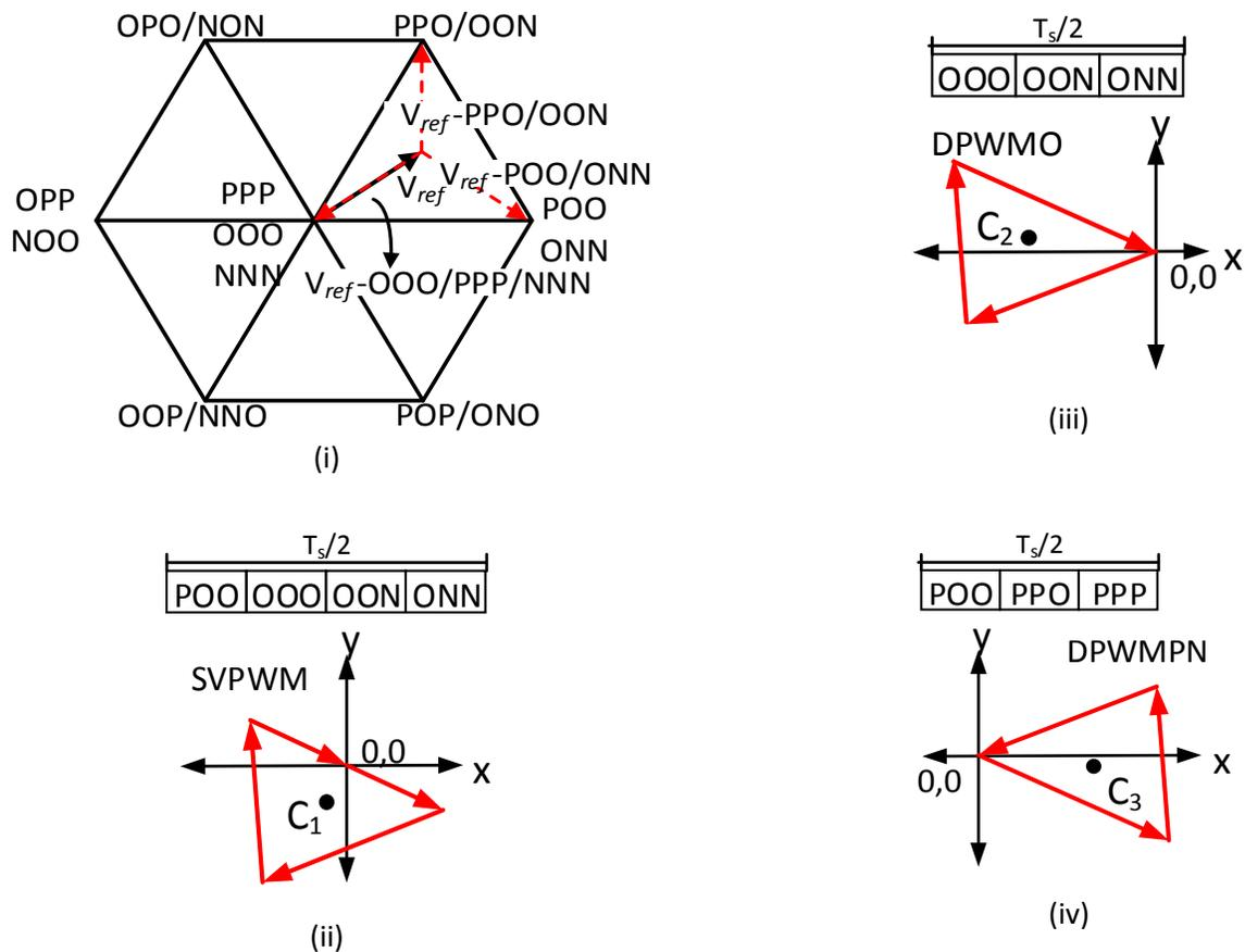
Figure 4-8. (i) Switching cycle voltage ripple, Switching cycle current ripple comparison between (ii) SVPWM, (iii) DPWMO, and (iv) DPWMPN
