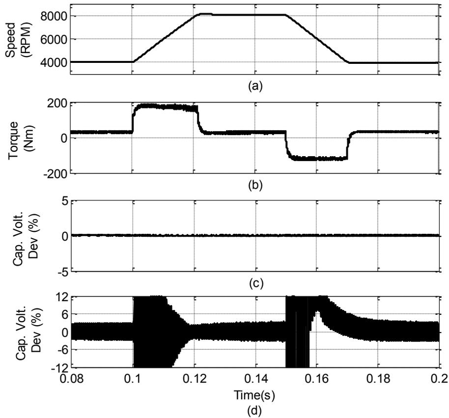
Figure 3-7. Transient Operation: (a) Speed Profile, (b) Torque profile, Capacitor voltage deviation with (c) dual T-NPC and (d) single T-NPC
