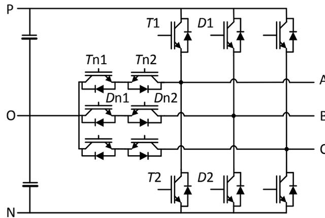
Figure 4-1. Three-level T-NPC inverter; showing the inner devices ( $T_{n1}$ - $D_{n1}$  and  $T_{n2}$ - $D_{n2}$ ) and outer devices ( $T_1$ - $D_1$  and  $T_2$ - $D_2$ )
