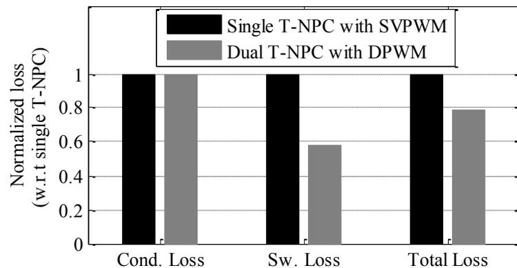
Figure 3-13. Loss reduction using Dual T-NPC topology due to absence of additional switching instances as in single T-NPC topology
