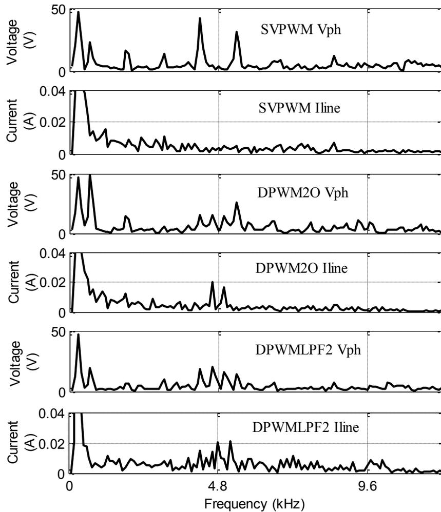
Figure 5-14. Experimental phase-DC-link neutral voltages' and line currents' harmonic spectra for SVPWM, DPWM20, and *DPWMLPF2* - experimental conditions (modulation index: 0.4, fundamental frequency: 200 Hz, switching frequency: 4800 Hz, power factor: 0.5, time step: 1 ms/div). Red rectangles show current peaks
