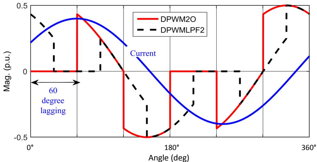
Figure 5-1. Phase difference between a-phase fundamental current (power factor 0.5) and average phase to DC-link neutral voltage waveforms for DPWM20 and DPWMLPF2
