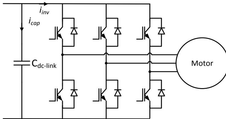
Figure 1-3. Conventional 2-level VSI and motor controlled based on the width, time-instants and frequency of the ON/OFF signal pulses that are fed to the gates of the inverter's switching devices. This topology has six IGBT-diode pair, and has highest switch-utilization (defined as the ratio of maximum output power to the maximum installed capacity of the inverter) [4] and lowest conduction loss amongst all inverters.
