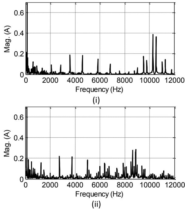
Figure 6-11. Output Current harmonic spectrum (i) without and (ii) with variable switching frequency PWM
