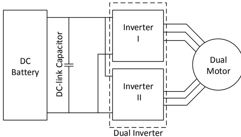
Figure 1-2: Dual Inverter Dual Motor topology
