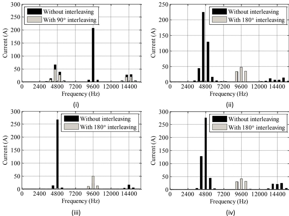
Figure 2-5. Capacitor harmonic spectrum for without and with interleaved PWM (i) m: 0.5 SVPWM with interleaving angle 90°; (ii) m: 1 SVPWM with interleaving angle 180°; (iii) m: 0.5 DPWM2 with interleaving angle 180°, and (iv) m: 1 DPWM2 with interleaving angle 180°
