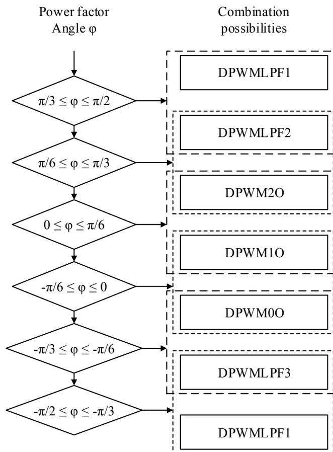
Figure 5-3. Combinations of the DPWMO sequences for generalized DPWMO (GDPWMO) based on operating power factor angle
