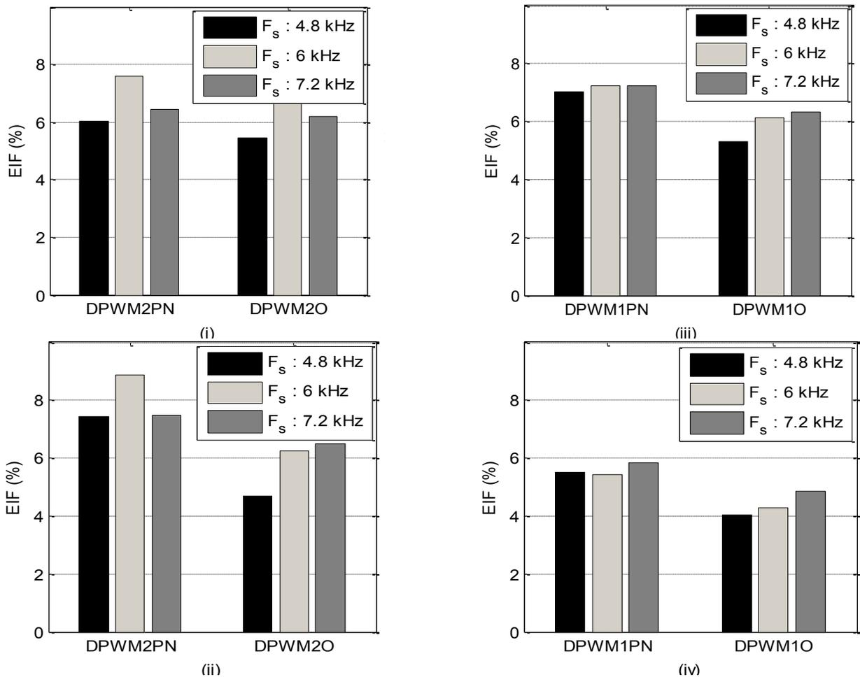
Figure 4-21. Experimental efficiency improvement factor (EIF) comparison between – (i) DPWM2PN and DPWM2O at 0.2 modulation index and 0.866 power factor, (ii) DPWM2PN and DPWM2O at 0.4 modulation index and 0.866 power factor, (iii) DPWM1PN and DPWM1O at 0.2 modulation index and 0.98 power factor, and (iv) DPWM1PN and DPWM1O at 0.4 modulation index and 0.98 power factor
