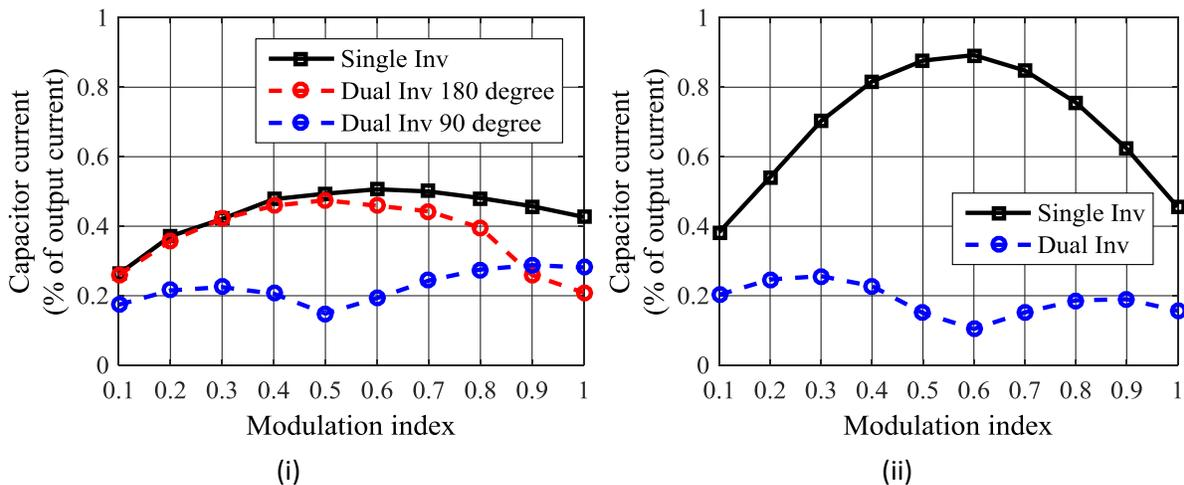
Figure 2-6. DC-link capacitor current w.r.t. RMS output current for (i) SVPWM, and (ii) DPWM2 strategies
