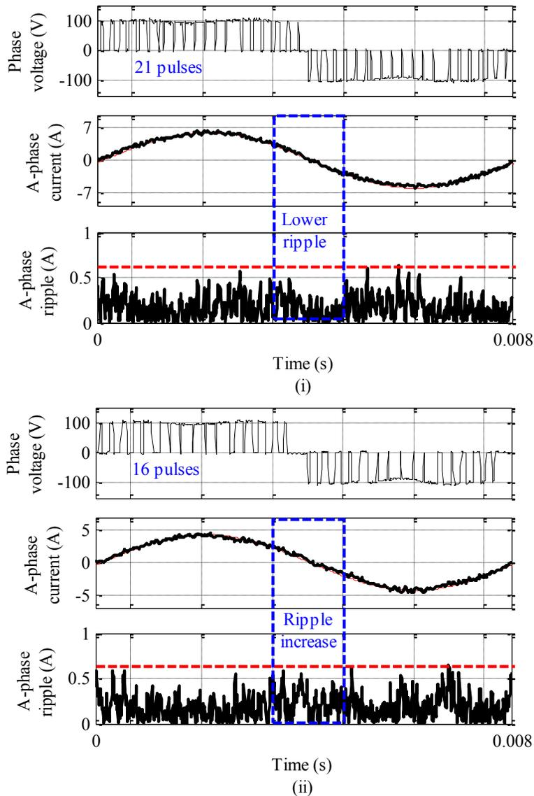
Figure 6-14. Comparison of experimental phase voltage, number of switching, current, and current ripple for SVPWM with (i) constant and (ii) variable switching frequency, Operating modulation index=0.95
