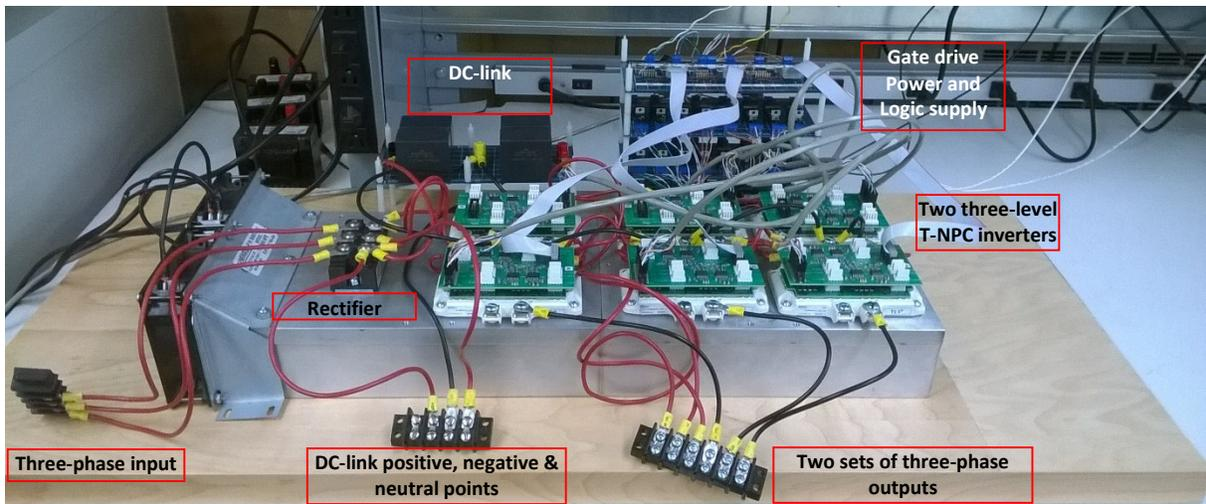
Figure Ap\_B-5: The experimental setup of dual T-type inverters
