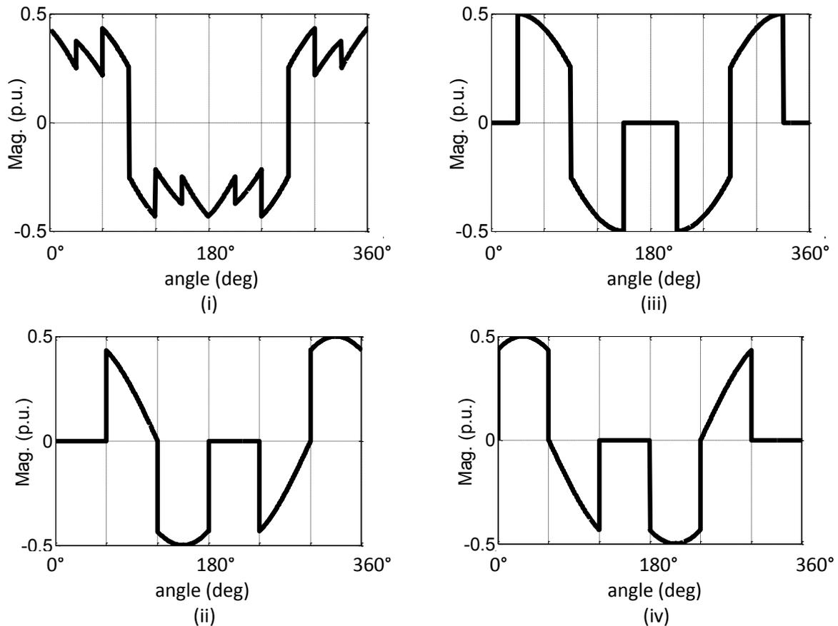
Figure 4-3. Average A-phase to DC-link neutral voltage waveforms for modulation index less than 0.5, normalized w.r.t DC-link voltage for conventional PWM templates - (i) SVPWM ; (ii) DPWM20; (iii) DPWM10; (iv) DPWM00 ; 0.5 signifies half DC-link voltage
