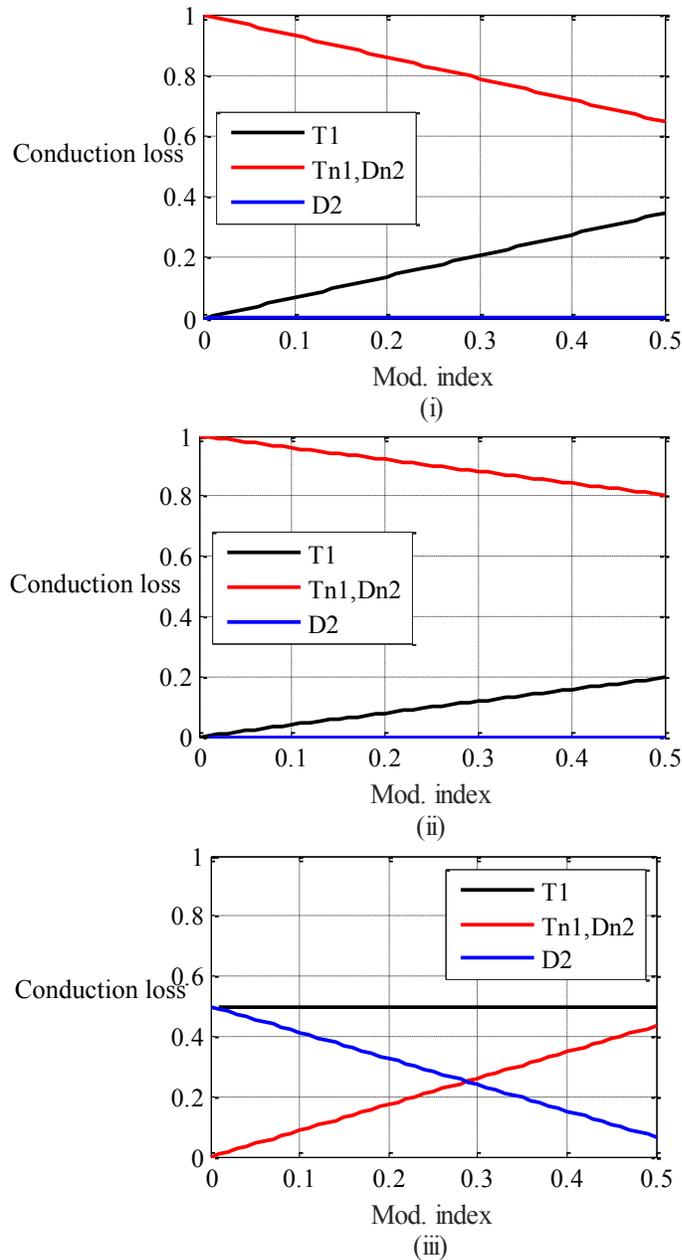
Figure 4-7. Device conduction loss comparison between (i) SVPWM, (ii) DPWM2O, and (iii) DPWM2PN over change in modulation index.
