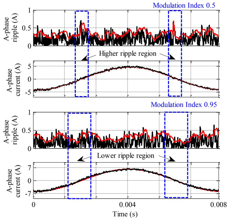
Figure 6-13. Experimental ripple variation of SVPWM at 0.5 and 0.95 modulation index
