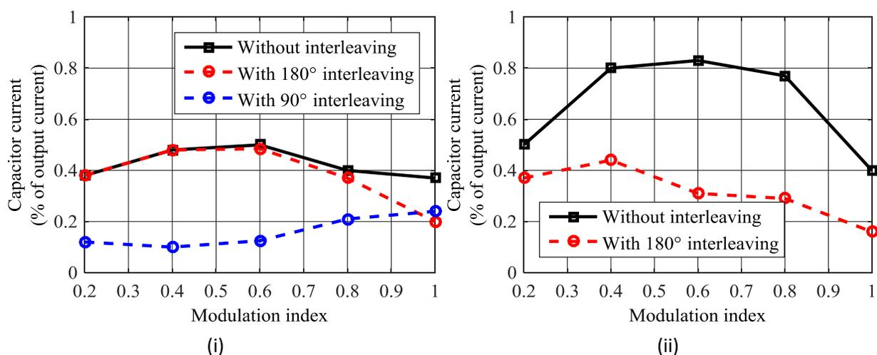
Figure 2-11. Experimental results - DC-link capacitor current w.r.t. RMS output current for (i) SVPWM, and (ii) DPWM2 strategies
