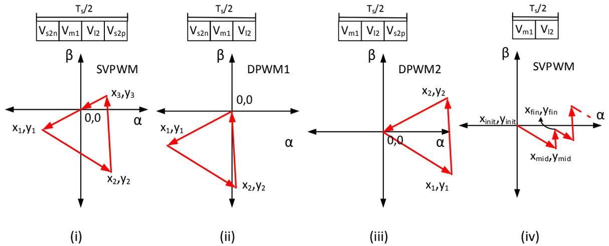
Figure 6-2. Current ripple trajectory in a PWM technique in subsector 4, sector I for - (i) Continuous SVPWM, (ii) Discontinuous PWM1, (iii) Discontinuous PWM2 and (iv) over-modulation region for SVPWM and DPWM strategies where short vectors are not used.  $T_s$  corresponds to one switching period
