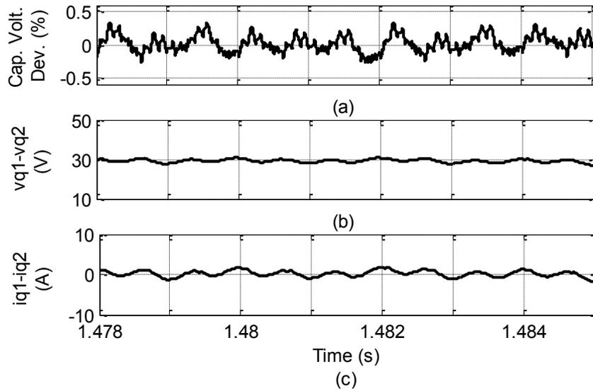
Figure 3-8. Operation with unbalance in winding impedance: (a) Capacitor voltage Difference, (b) q-axis voltage difference, (c) q-axis current difference
