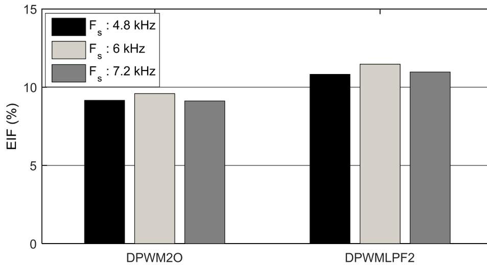
Figure 5-15. Experimental efficiency improvement factor (EIF) using DPWM2O and DPWMLPF2 in comparison to conventional SVPWM strategy at 0.4 modulation index and 0.5 power factor
