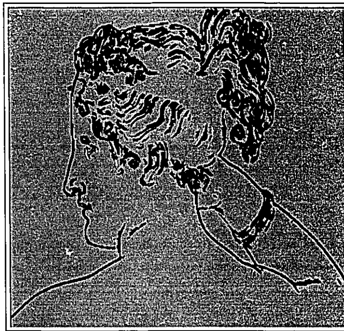
FIGURE 4.18. The line drawing provides sufficient information to humans to allow them to recognize some scenes. This line drawing was extracted from the gray-level image with Iverson's logical-linear operators for edges and lines [66].
