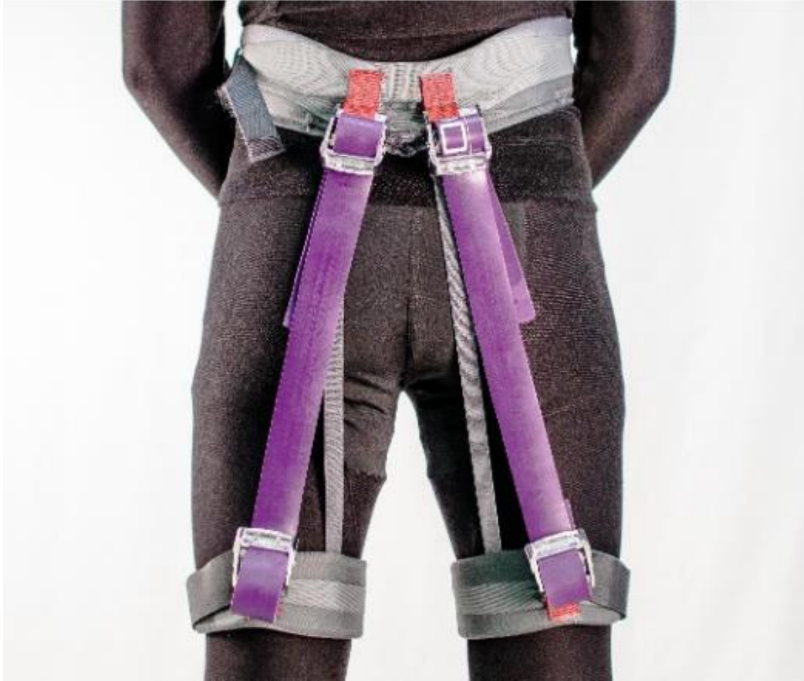
Figure 1. The posterior view of the exotendon system employing the stiffest elastic condition (STAP).
