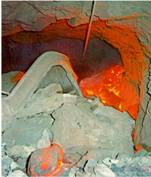
Figure 1.1: Underground sulphide mine fire in Kimberly, BC (CIM Bulletin, 1977)
