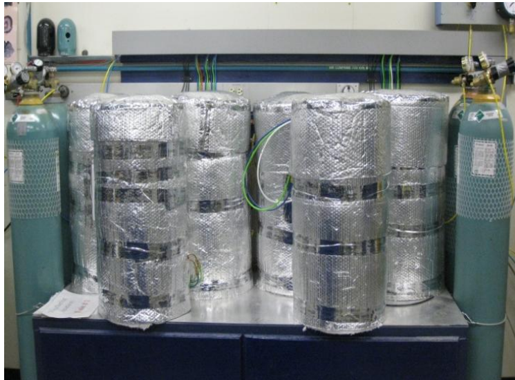
Figure 3.6: Weathering apparatus setup
