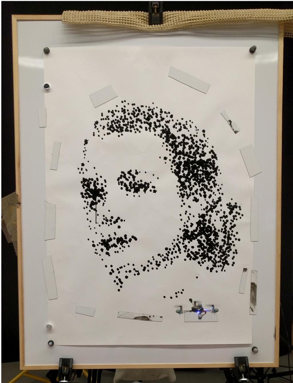
Figure 7-3: A photo of our largest print with 2000 stipples in the process of being drawn on a 100 cm × 70 cm canvas.
