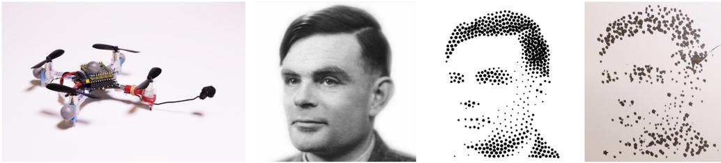
Figure 1–1: Our stippling aerial robot uses motion capture markers for positioning, and an ink sponge on a small arm to create stipples. Also shown is an example result: from left to right, a well known image of Alan Turing, a stippled version of the image with 500 dots, and a finished print with 500 stipples, drawn using a dynamic correction for the placement of stipples.
