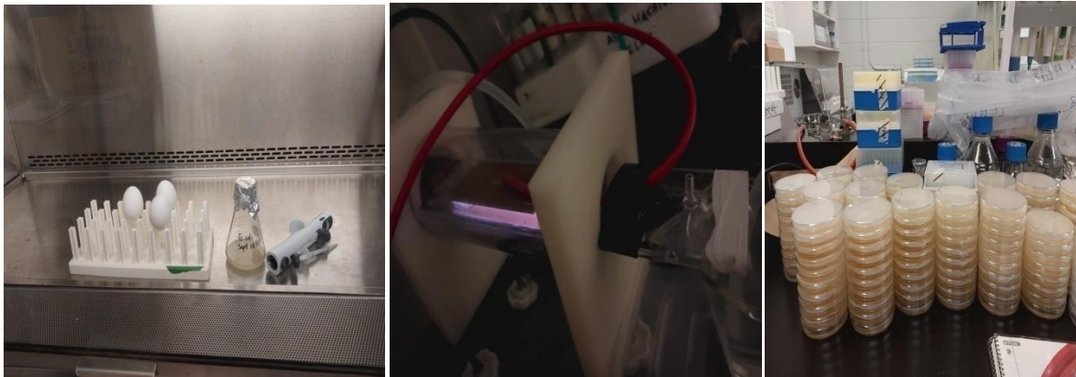
Figure 3.3 (a) eggs contaminated with E. coli (b) PAW treatment (c) Plating after serial dilution.
