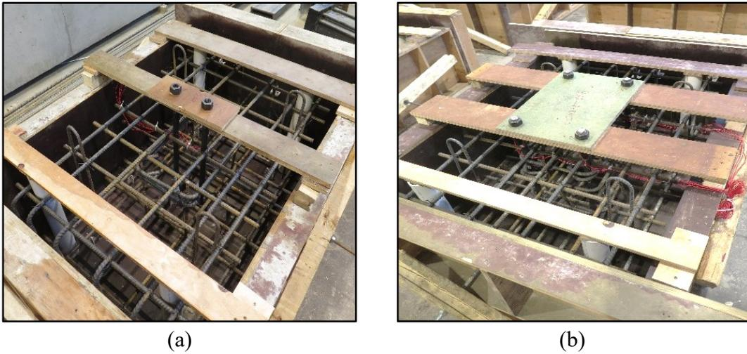
Figure 3.9: Formwork and steel cages prior to casting: (a) 2-AR and (b) 4-AR
