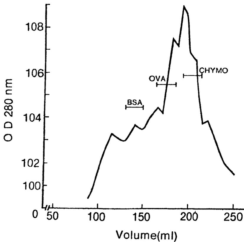
Figure 12. Elution profile of normal urinary protein sieved on molecular sieve chromatography Sephadex G-75 superfine. Elution recorded at 280 nm, (P44 corresponding to elution volume of ovalbumin) and P25 (corresponding to elution volume of chymotrypsinogen) were collected separately and concentrated.
