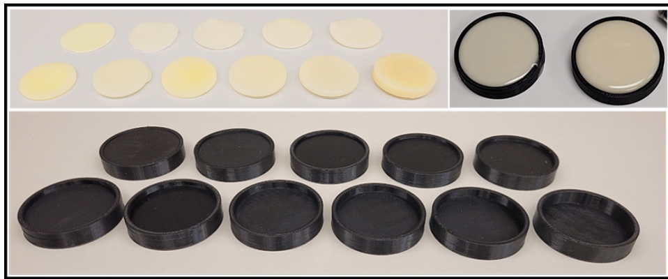
Fig. 7.1: Fabricated skin phantoms with thickness varying 0.5 – 5 mm with 0.5 mm increments and 8 mm thick control skin phantom (top left), 3D printed cylindrical molds (bottom) and skin mimicking material poured into 3D printed molds at final fabrication step (top right).
