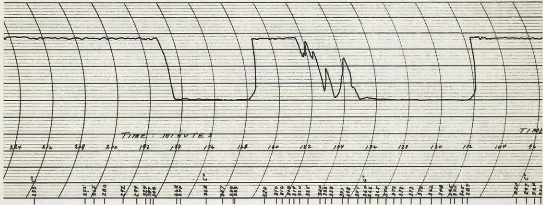
B- RECORD OBTAINED WITH CURIE POINT METER FOR A SAMPLE OF PYRRHOTITE
