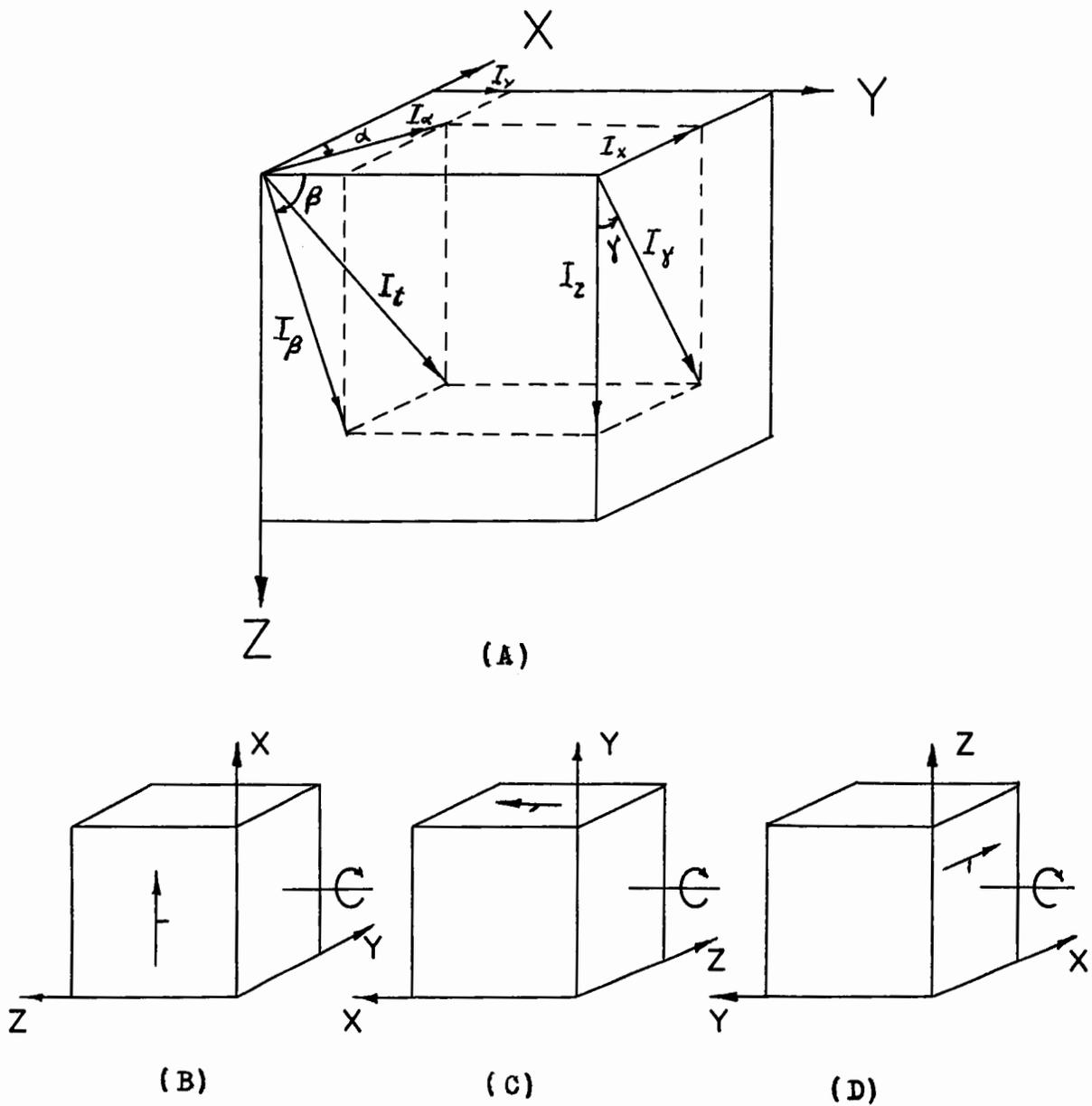
Fig. 4 - Nomenclature Diagram (A); Spinning positions to measure  $I_\alpha$  and  $\alpha$  (B),  $I_\beta$  and  $\beta$  (C),  $I_\gamma$  and  $\gamma$  (D).
