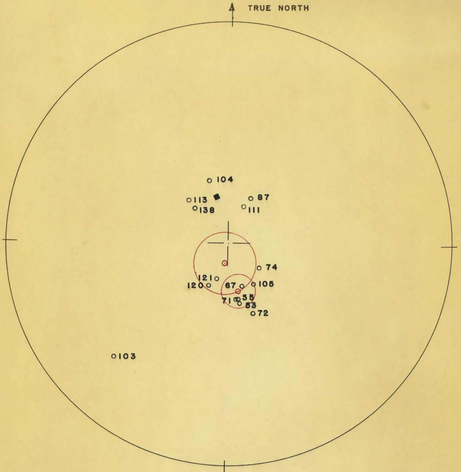
Fig. 11 : Stereographic Projection of Magnetization Vectors for 15 samples from Yamaska Mountain, after Magnetic Washing.
