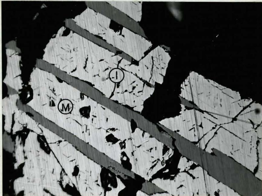
F- Specimen No. 105: Photomicrograph of opaque mineral grain showing exsolution lamellae of ilmenite (I) from magnetite (M); magnification X 400.
