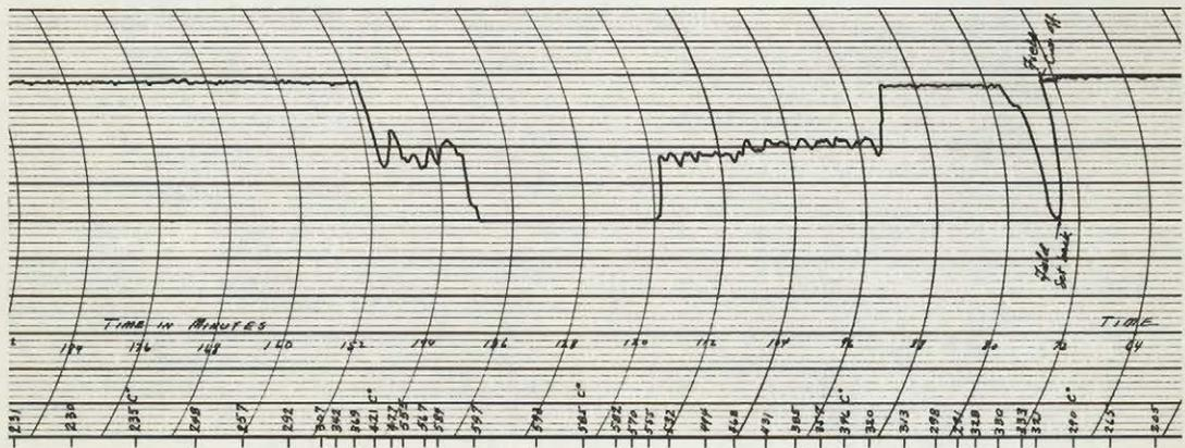
C- RECORD OBTAINED WITH CURIE POINT METER FOR A SAMPLE COMPOSED OF PART OF THE MAGNETITE AND PYRRHOTITE USED FOR A- AND B-
