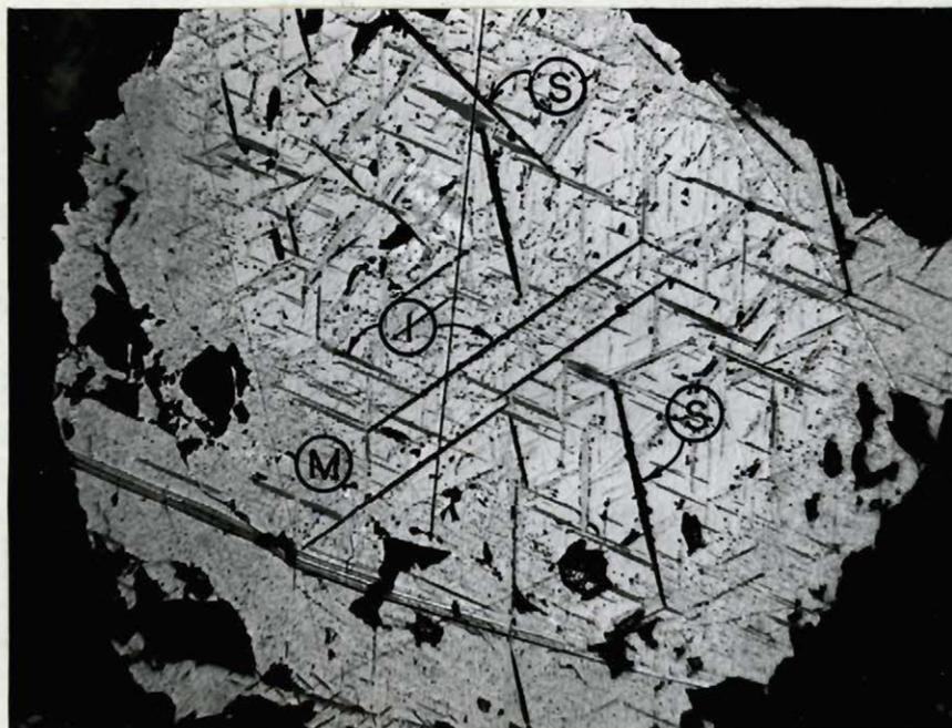
C- Specimen No. 42: Photomicrograph of opaque mineral grain showing exsolution lamellae of ilmenite (I) from magnetite (M) and MgAl Spinel (S) intergrowth; magnification X 400.
