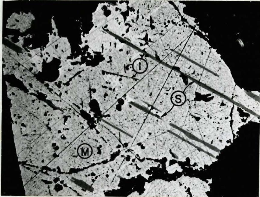
A- Specimen No. 37-B: Photomicrograph of opaque mineral grain showing exsolution lamellae of ilmenite (I) from magnetite (M) and MgAl Spinel (S) intergrowth; magnification X 400.
