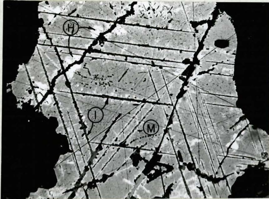
E- Specimen No. 74: Photomicrograph of opaque mineral grain showing exsolution lamellae of ilmenite (I) from magnetite (M) and oxidation of magnetite into hematite (H) along fissures; magnification X 400.
