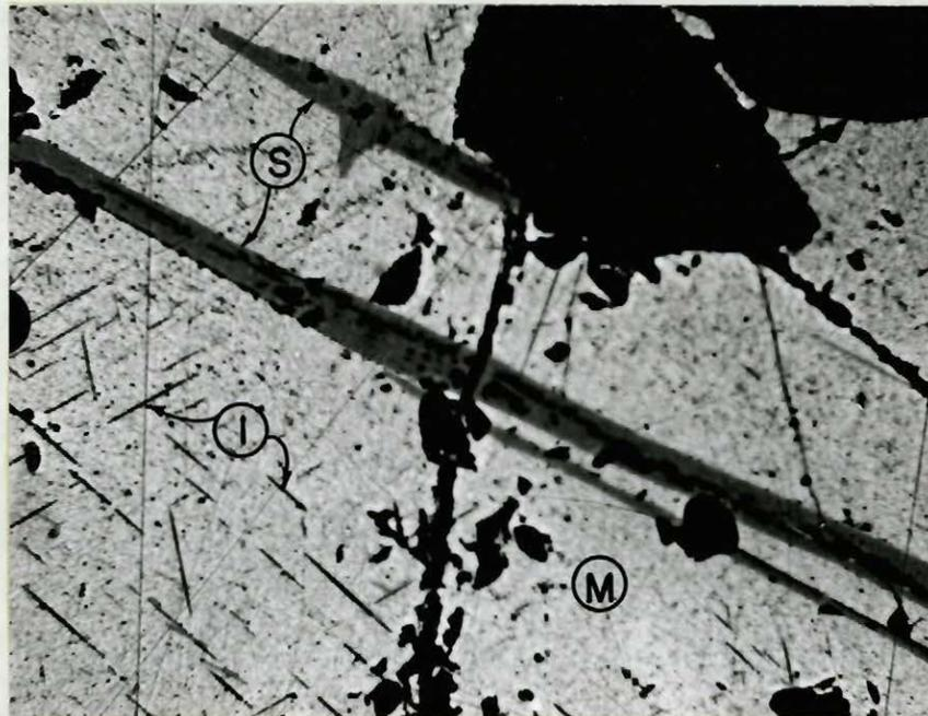
B- Specimen No. 38: Photomicrograph of opaque mineral grain showing exsolution lamellae of ilmenite (I) from magnetite (M) and MgAl Spinel (S) intergrowth; magnification X 400.
