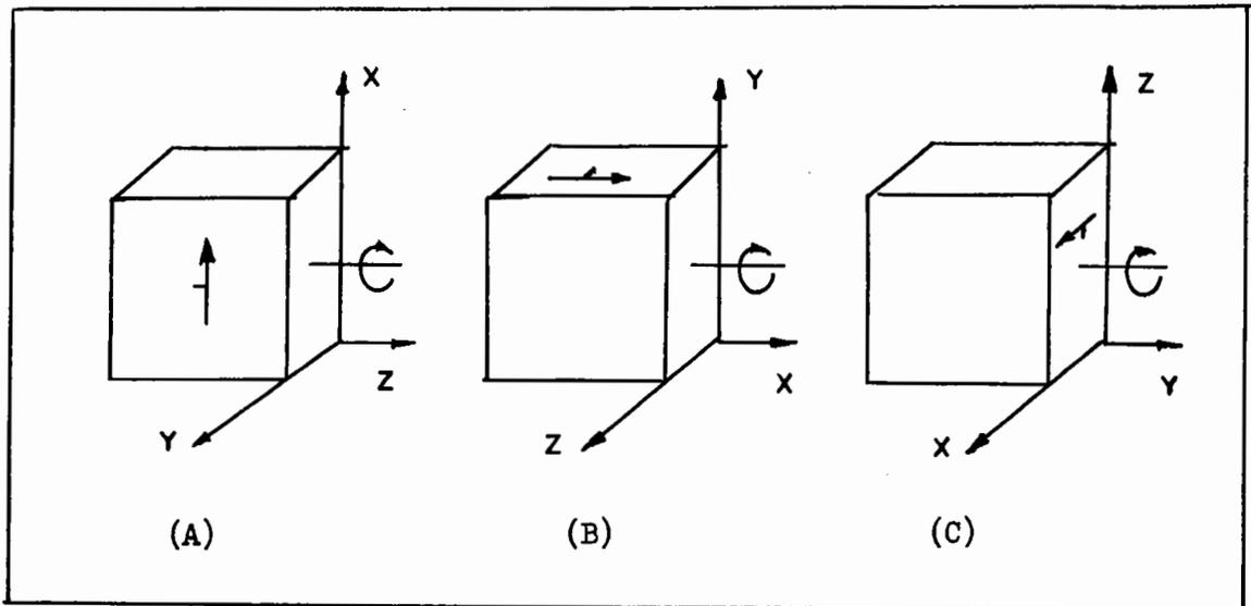
Fig. A-2: Cube positions for the measurements of  $\alpha'$ (A),  $\beta'$ (B) and  $\gamma'$ (C).
