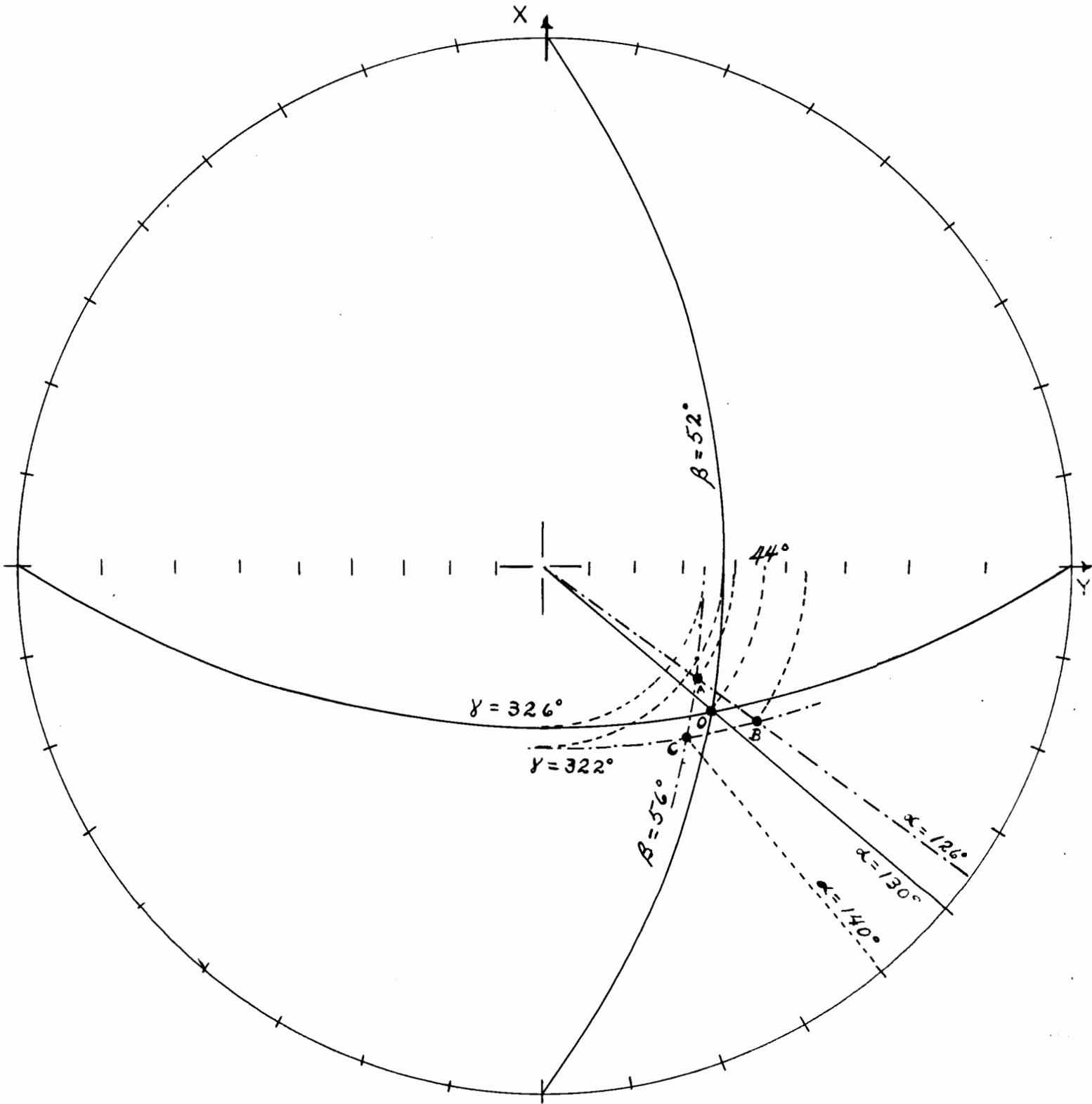
FIG. A-1: EXAMPLE OF DECLINATION AND INCLINATION DETERMINATION
