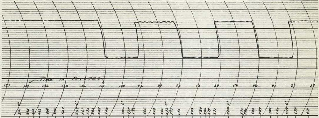
A- RECORD OBTAINED WITH CURIE POINT METER FOR A SAMPLE OF MAGNETITE
