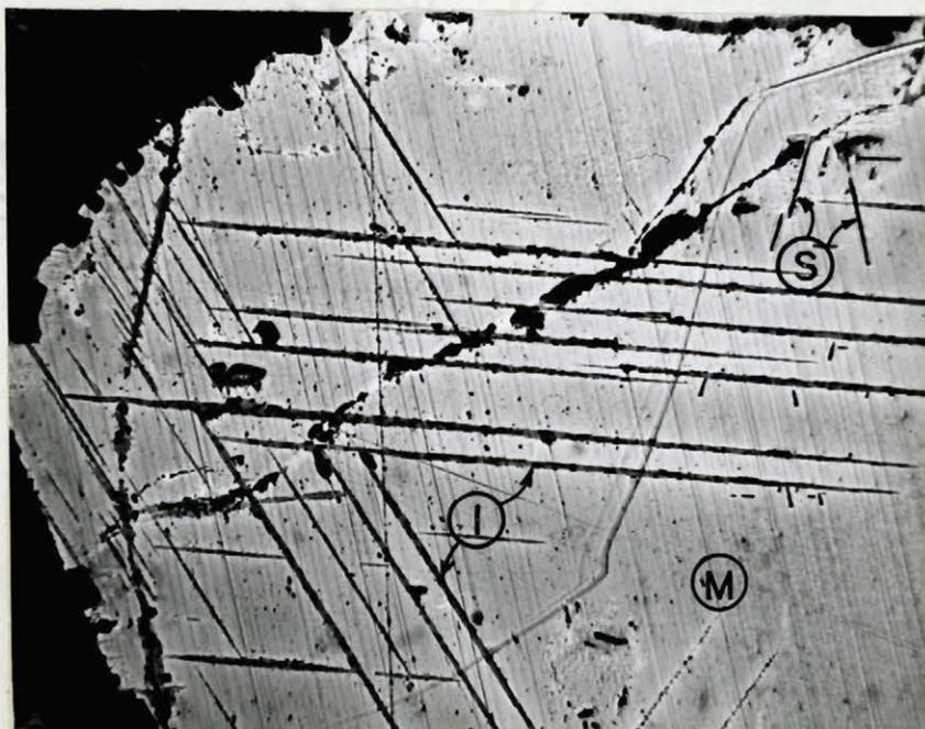
D- Specimen No. 71: Photomicrograph of opaque mineral grain showing exsolution lamellae of ilmenite (I) from magnetite (M) and MgAl Spinel (S) intergrowth; magnification X 400.
