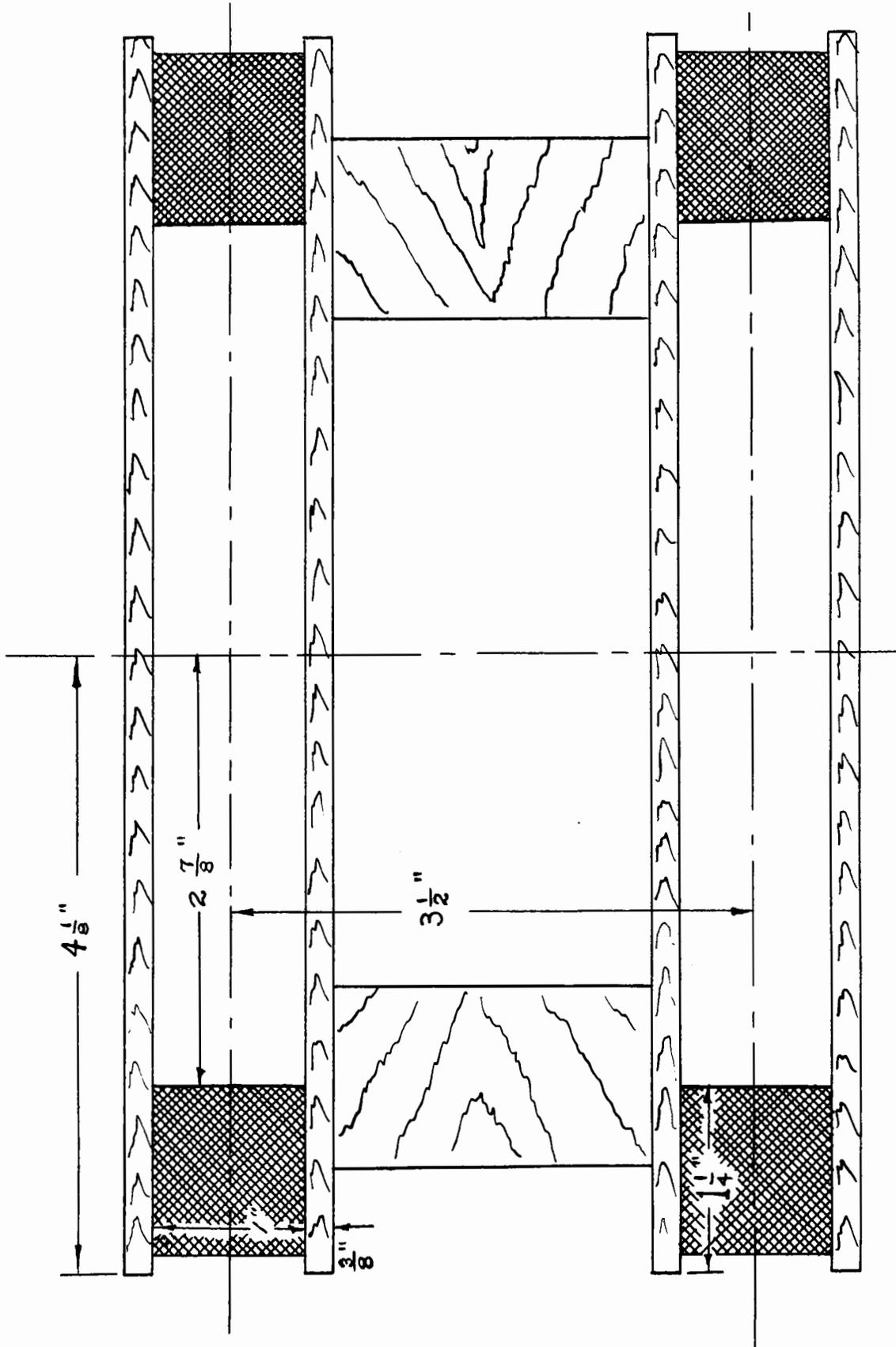
FIG. 10: DEMAGNETIZING COIL DESIGN
