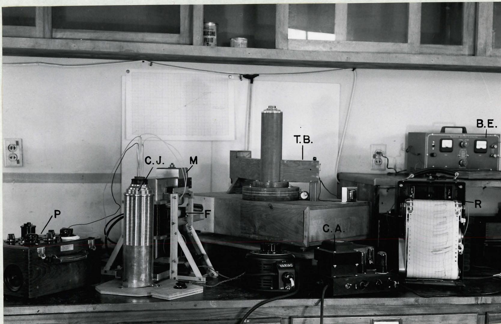
Fig. 14: CURIE POINT METER ASSEMBLAGE
