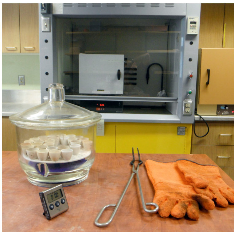
Figure 5.4 Crucibles cooling in the desiccator with the muffle furnace in the background under the fume hood.
