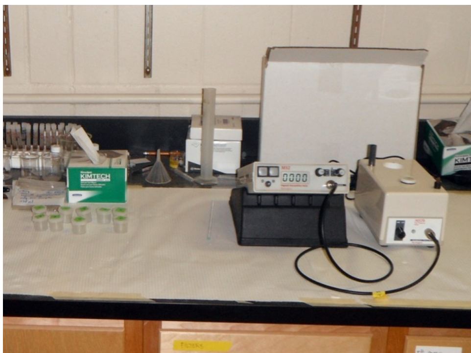
Figure 5.2 Measuring magnetic susceptibility using a Bartington MS2B sensor.
