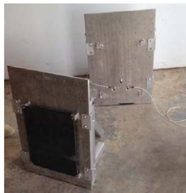
(b) Intelligent obstacles shown with protective shield (left) and sensors exposed (right)
