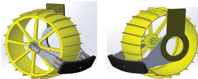
Figure D-1: CAD model of bumper assembled on RCP wheel
