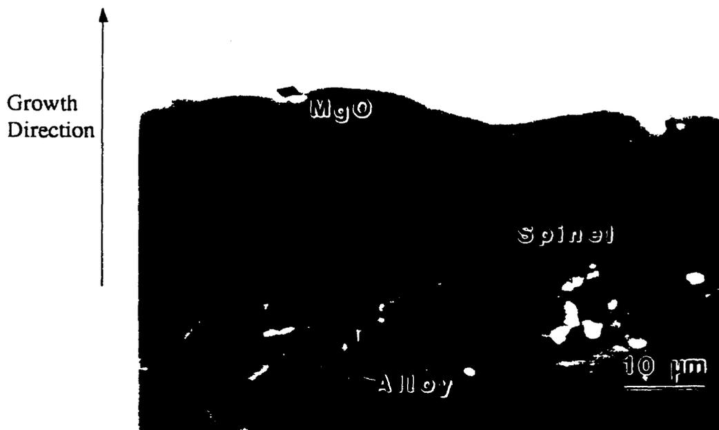
Fig. 5.16: Cross-section of the alloy showing the formation of surface oxides on a (0/3) alloy (15 hours).
