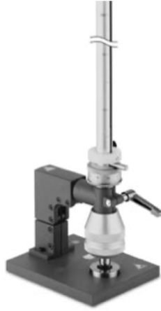
Figure 2.3 Falling weight impact test apparatus.
