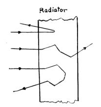
the radiator which the scattered particles traverse and while doing so they will lose velocity just as has been shown to be the case whenever (3-rays pass through matter. It is evident, then, that the real range of the scattered rays is the range actually found plus the equivalent of the average path in the radiator. It is not impossible, though it cannot yet be stated definitely, that this completely explains the
