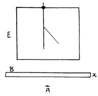
The active material is placed at A and the ionization is measured by the rate of fall of the gold-leaf in the electroscope E. The absorbing plate B, of thickness x, is placed in the position as shown, and the ionization measured as before. The ionization, and hence the intensity, is found to decrease
