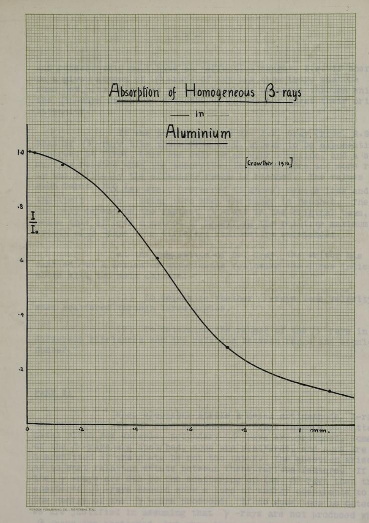
and consequently must have an "effective range", i.e. if there be a given stream of (3-rays of any one type there must be some definite thickness of any absorbing material through which the (3-rays cannot be detected no matter how great their original intensity.
