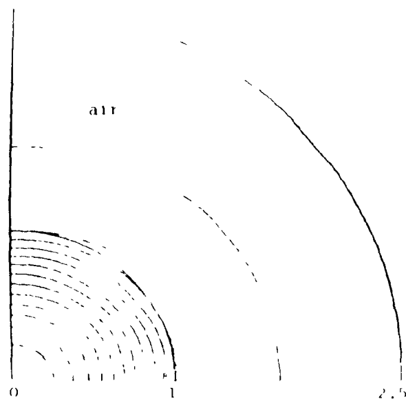
Fig. 7 - Dielectric rod, H_x field, linear scale, \gamma = 1.450 , fundamental mode. ( H\Gamma_{11} ) ( F_y and S_z are similar )
