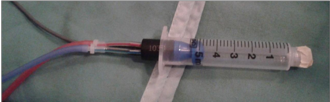
Figure 5-2: Artificial cavity consisting of a 5-ml syringe. The OAE probe is inserted into the lumen; here it is shown at the 5-ml position.
