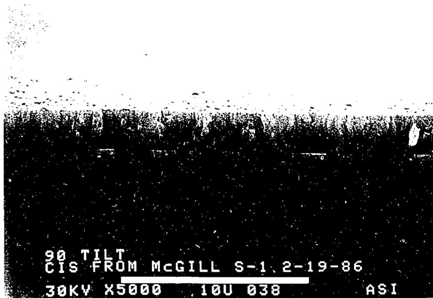
Fig. 3.3 An SEM micrograph of a fractured CuInSe<sub>2</sub> film deposited on a Mo/glass substrate showing a uniform CuInSe<sub>2</sub> thickness.
