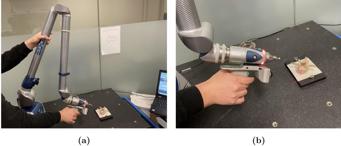
**Figure 3.16:** The *FARO Arm* with laser line probe attached to the end effector for 3D scanning.
