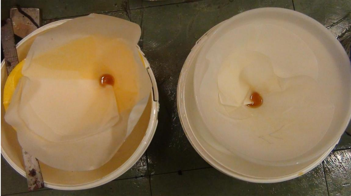
Figure 4.03. Attached Watman-5 filter paper in the SEN in order to collect entrained slag
