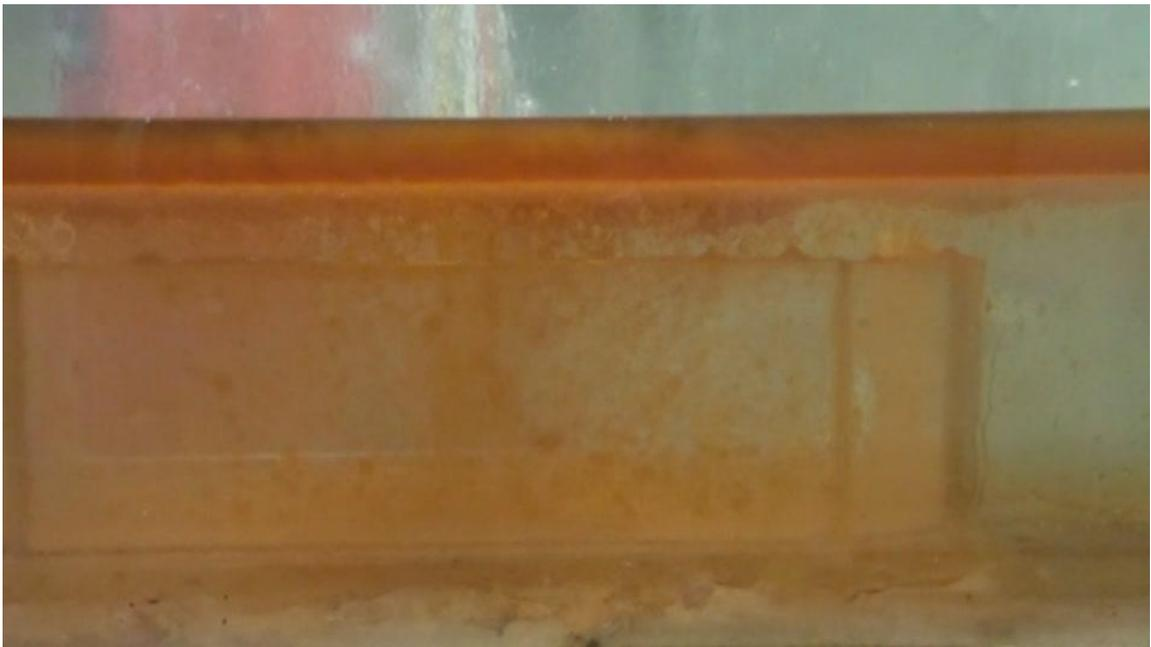
Figure 4.05. Slag movements in a tundish fitted with a MIIP during a ladle change operation
