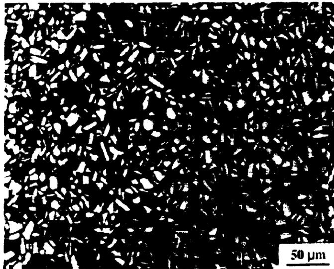
Figure 2. Microstructure of Duralcan 6061/Al<sub>2</sub>O<sub>3</sub>/40p metal-matrix composite
