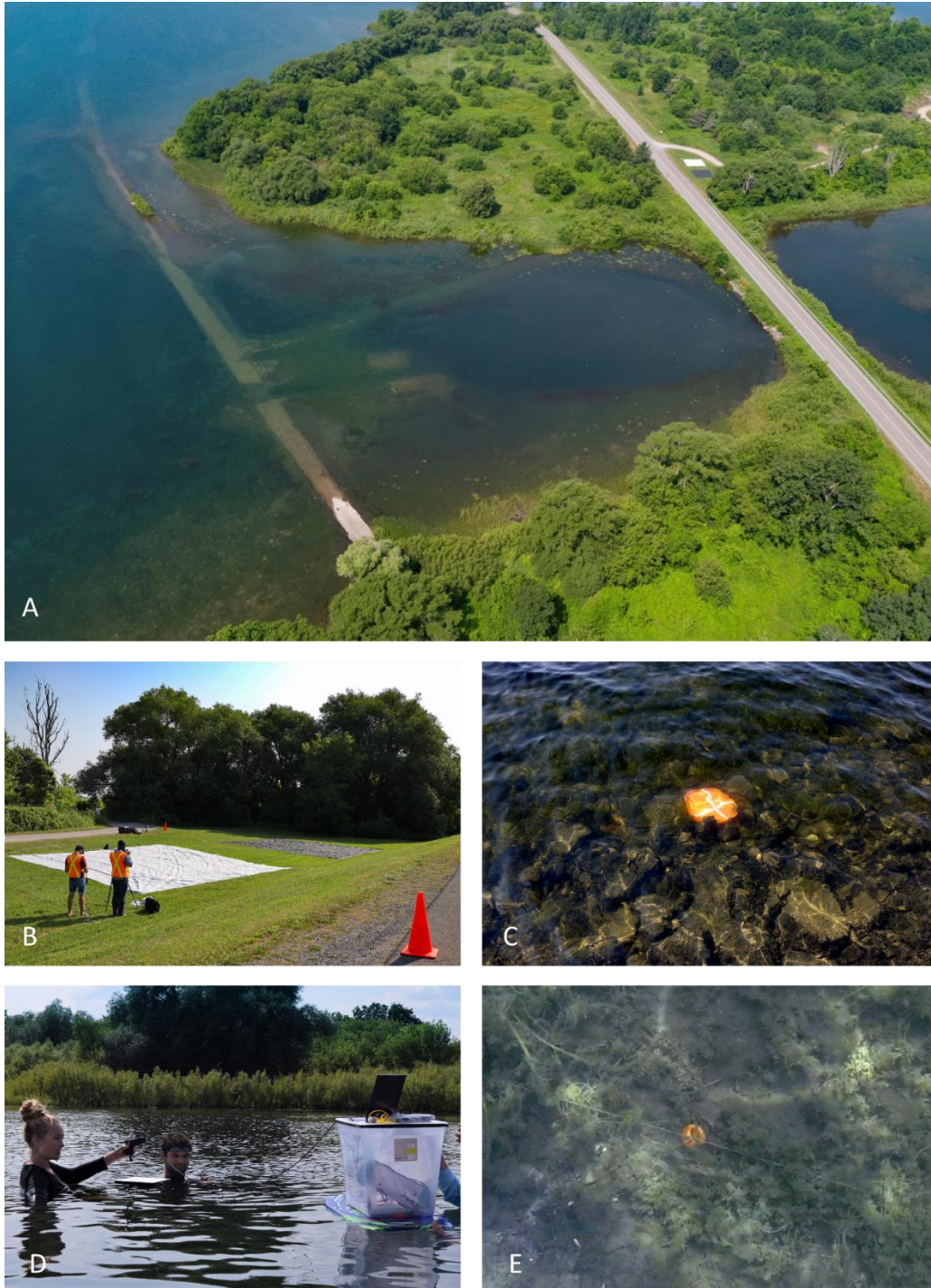
Figure SM3.1. Experimental field set up. A) RPAS photo of the site acquired the same day (07/26/2019) as the CASI HSI; B) reference target set up for verifying the atmospheric compensation of the CASI HSI, targets are two tarpaulins with known reflectance; C) GCP placed at the site for orthorectification of the RPAS images and orthomosaic; D) improvised floating platform for underwater ASD measurements, measurement of Spectralon reference panel at the water's surface is shown here; E) example transect marker captured in video footage (this point would have been labeled as Chara sp.).
