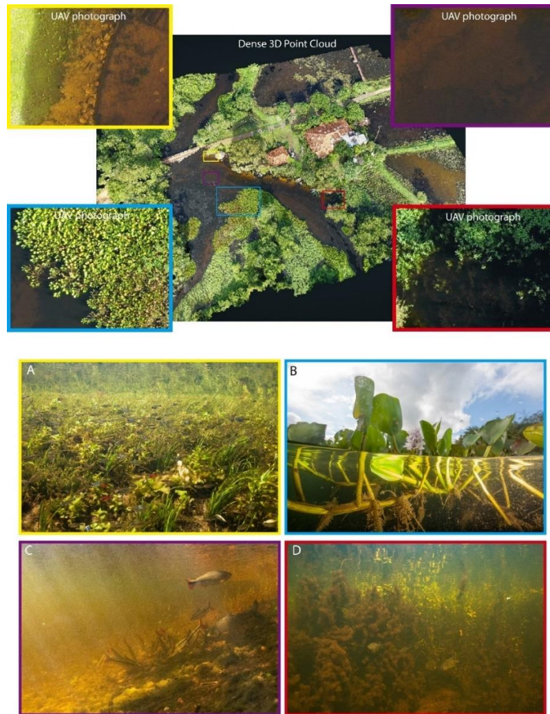
Figure 2.14. Dense 3D point cloud from the Salobra river, Mato Grosso do Sul, Brazil generated through a Structure-from-Motion Multiview Stereo workflow from 768 UAV photographs. Photographs were acquired with a DJI Mavic 2 Pro UAV with an integrated Hasselblad L1D-2C camera. The camera has a 1" sensor (77° field of view) producing an image size of 5472 × 3648 pixels. A median of 67,753 key points were found per photograph with a median of 13,416 matches per photograph. Final ground sampling distance of the model is 1.2 cm. Extensive floating water hyacinth ( Eichhornia crassipes ) can be seen. The interactive point cloud can be accessed at https://bit.ly/waterhyacinth3D . Panel A (yellow) illustrates a shallow (<30 cm) area with several species of SAV which produce a habitat utilized by small characins. Panel B (blue) illustrates floating E. crassipes in deep (>2 m) water frequented by giant otters ( Pteronura brasiliensis ) and caimans ( Caiman yacare ). Panel C (purple) is a mid-range depth (1–2 m) with large patches of algae on the substrate. This open water habitat is frequented by larger fish species such as Prochilodus lineatus . Panel D (red) shows a bed of Camboba sp. in deep water (>2 m). The dense stems provide habitat for species such as Pygocentrus nattereri and Serrasalmus maculatus .
