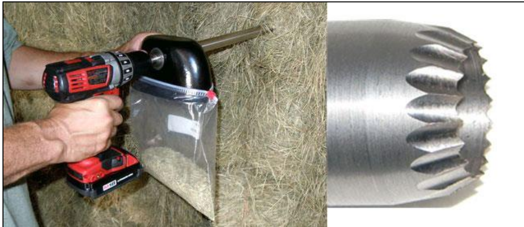
Figure 4 - Hay Bale Corer for Sampling (RDS Coleman Consulting, 2011)
