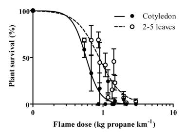
Figure 3.4. Response of barnyardgrass seedlings with one leaf to greater-than-four leaves to a single flame weeding treatment. Flame doses ranged from 0.54 to 2.95 kg propane km<sup>-1</sup>. Weed response measured as percent of plants that survive flame weeding, as determined one to three days following flame treatment. Points represent mean values of data from four experiments in 2005 and three experiments in 2006. Error bars represent one standard error of the mean (SE).
