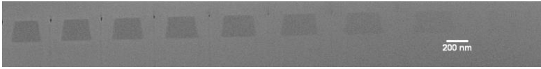
Fig. 3.8 Cross-section image of the voids when the grating size and spacing are 316 nm and 293 nm wide, respectively.
