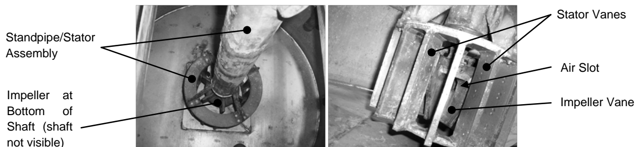
Figure 3.2 View of impeller/stator located at bottom of shaft near cell bottom (left image). Close-up of impeller/stator. Note air slot located between impeller vanes (right image)
