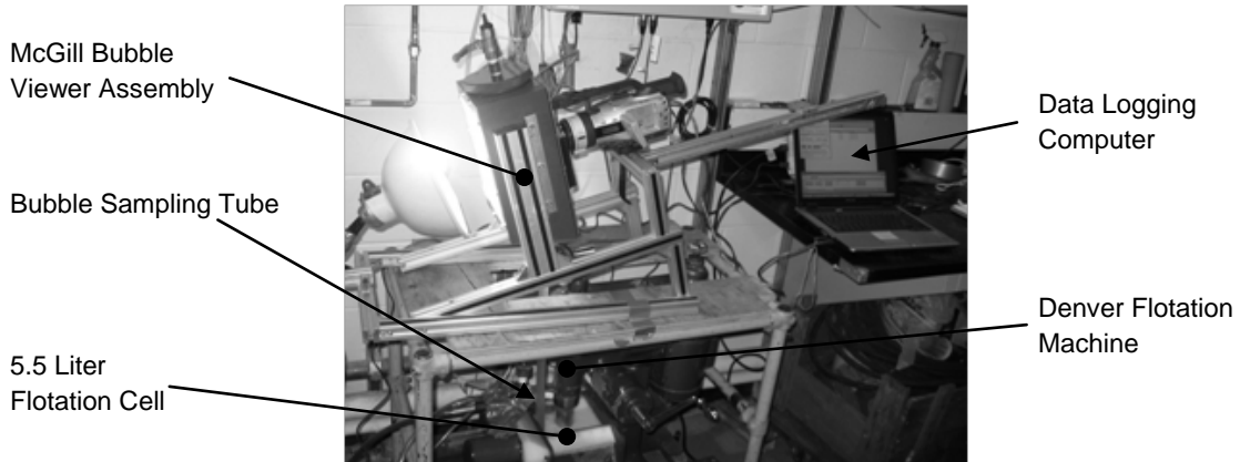
Figure 3.6 Arrangement of the Denver flotation machine and McGill Bubble Viewer positioned on stand above the cell. Note the bubble sampling tube extending down into the corner of the cell
