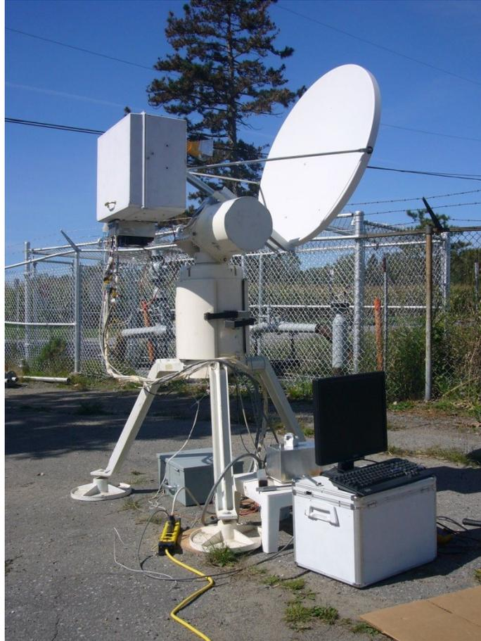
*Figure 1.3 The McGill Mesoscale Radiometer.*
