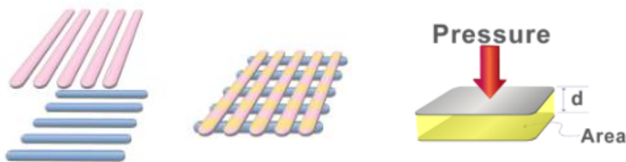
Figure 2.19 Capacitive technology based tactile sensors (PPS)
