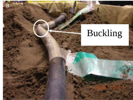
Figure 2.13 Tactile sensing sheets around deformed pipelines (Choo et al., 2007)
