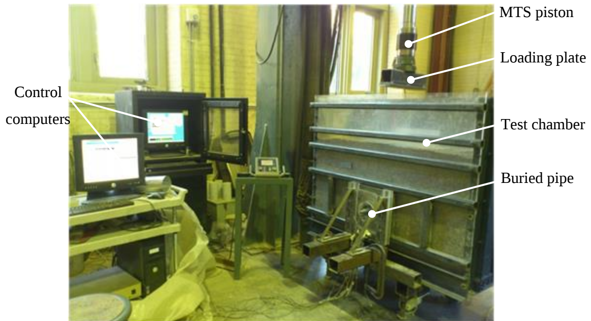
Figure 3.5 Details of the experimental setup
