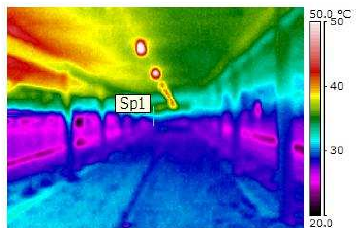
Figure 5.4: Infra-red view of the floor 1 inside barn B on February 18 th , 2009, in the absence of birds but with the solar air pre-heaters (left) and the ventilation system (right) in operation. The high temperature at the ceiling on the left side is created by the heater (left) in operation. A 10°C difference in air temperature is observed between the ceiling and floor, explaining the conductive heat exchange between floors.
